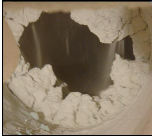
Fig 16: Ring formation in cement kiln
