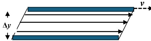
Fig 1.1: Definition of viscosity
