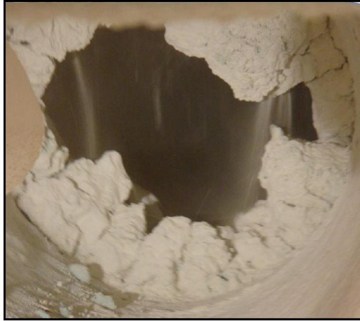
Fig 9.9 Ring formation in cement kiln
