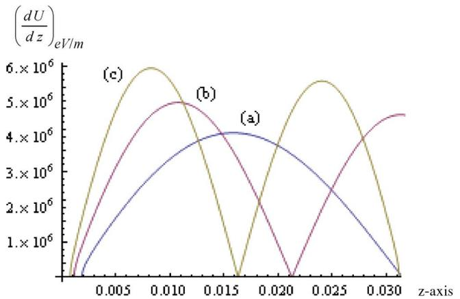
Fig. 7. Variation of the energy gradient along the  $z$ -axis for different microwave frequencies of (a) 3, (b) 4, and (c) 5 GHz, with a microwave intensity of  $5 \times 10^4 \text{ W/m}^2$ . The other parameters are the same as in Fig. 1.
