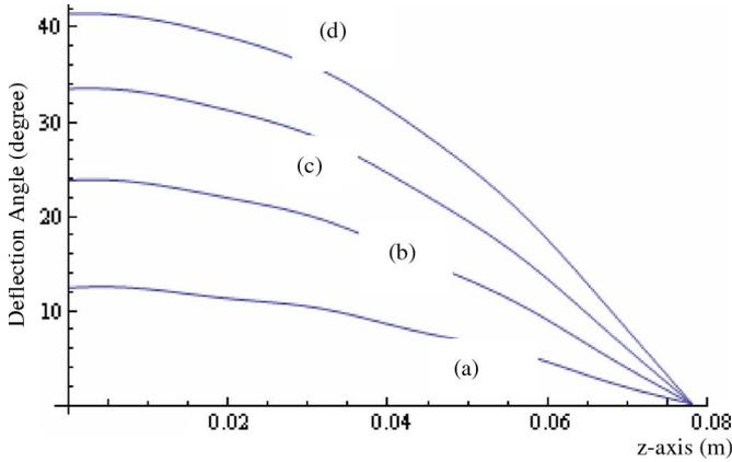
Fig. 1. Variation of the deflection angle along the  $z$ -axis for different microwave intensities of (a)  $10^4$ , (b)  $2 \times 10^4$ , (c)  $3 \times 10^4$ , and (d)  $4 \times 10^4$   $\text{W/m}^2$  with microwave frequency  $f = 2$  GHz, helical magnetic field of 0.1 T, and electron kinetic energy of 140 keV.
