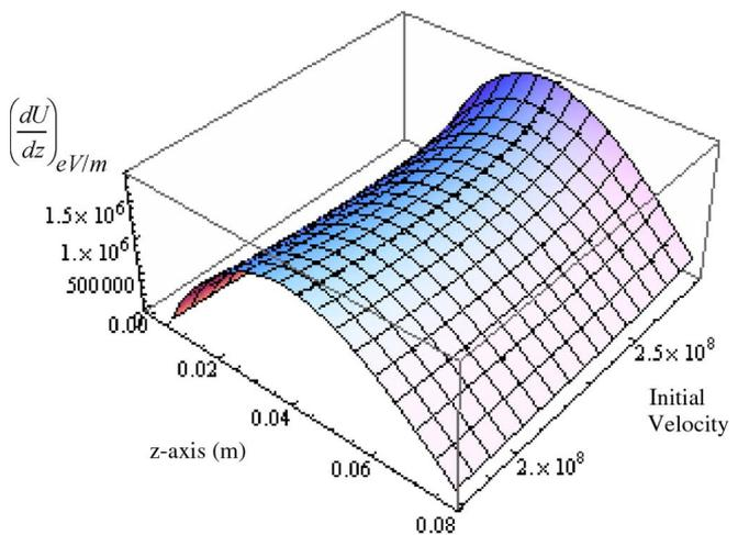
Fig. 8. Effect of the initial energy of the electron on the energy gradient along the  $z$ -axis with a microwave intensity of  $3 \times 10^4 \text{ W/m}^2$ . The other parameters are the same as in Fig. 1.
