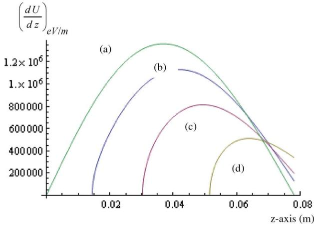
Fig. 9. Variation of the energy gradient along the  $z$ -axis for different helical magnetic fields  $B_0$  of (a) 0, (b) 0.1, (c) 0.2, and (d) 0.3 T, with a microwave intensity of  $3 \times 10^4$  W/m<sup>2</sup>. The other parameters are the same as in Fig. 1.
