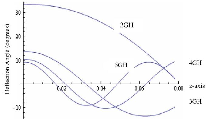
Fig. 2. Variation of the deflection angle along the  $z$ -axis for different microwave frequencies with a microwave intensity of  $3 \times 10^4$   $\text{W/m}^2$ . The other parameters are the same as in Fig. 1.
