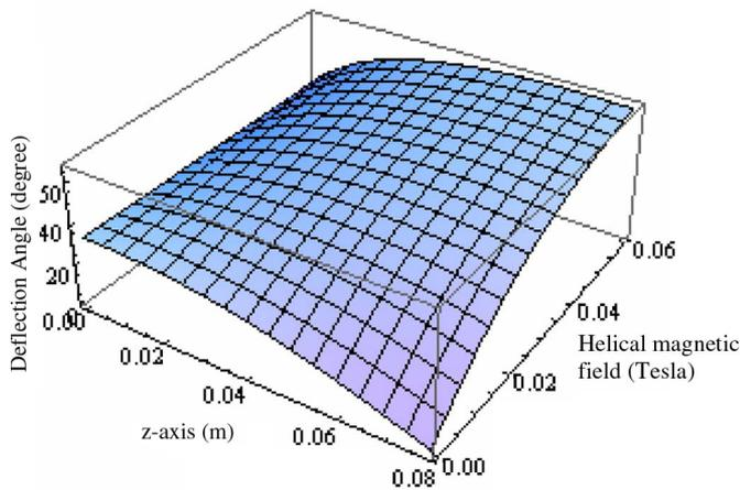
Fig. 5. Effect of the helical magnetic field on the deflection angle along the  $z$ -axis with a microwave intensity of  $3 \times 10^4 \text{ W/m}^2$ . The other parameters are the same as in Fig. 1.
