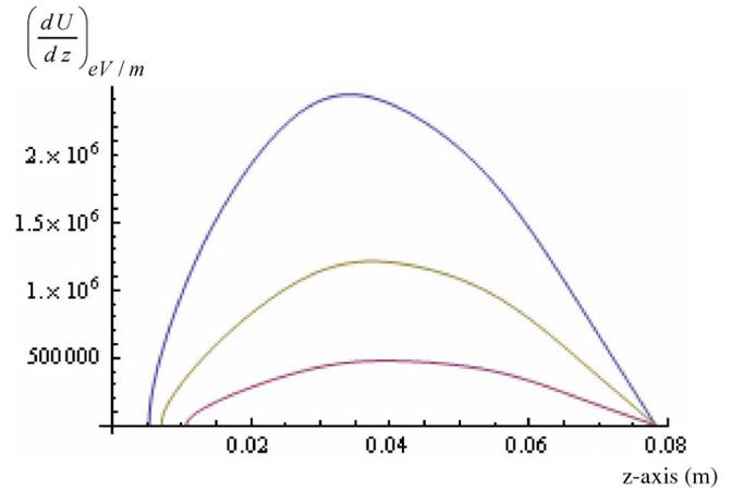
Fig. 6. Variation of the energy gradient along the  $z$ -axis for different intensities of the microwave of (a)  $10^4$ , (b)  $2 \times 10^4$ , and (c)  $4 \times 10^4 \text{ W/m}^2$ . The other parameters are the same as in Fig. 1.
