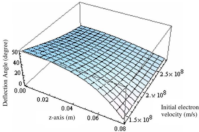
Fig. 4. Effect of the initial kinetic energy of the electron on the deflection angle along the  $z$ -axis for a microwave intensity of  $3 \times 10^4 \text{ W/m}^2$ . The other parameters are the same as in Fig. 1.
