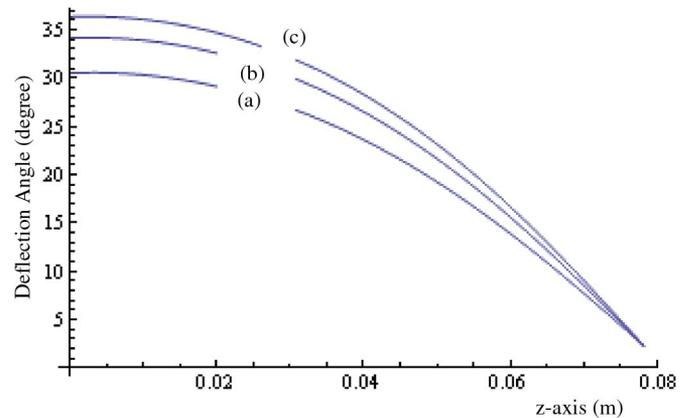
Fig. 3. Deflection angle along the  $z$ -axis at different points of injections of (a)  $3a/4$ , (b)  $a/2$ , and (c)  $a/4$  with a microwave intensity of  $3 \times 10^4$   $\text{W/m}^2$ . The other parameters are the same as in Fig. 1.
