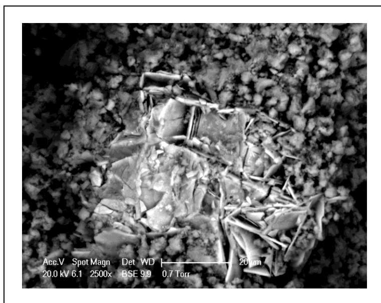
Figure 5. ESEM image of \text{TiO}_2 anatase polymorph in the red pigment sample (2500x, scale bar = 20 \mu\text{m} ).
