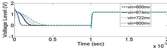
Figure 8. Output wave form of starved inverter at different input voltage in case of 2-bits.
