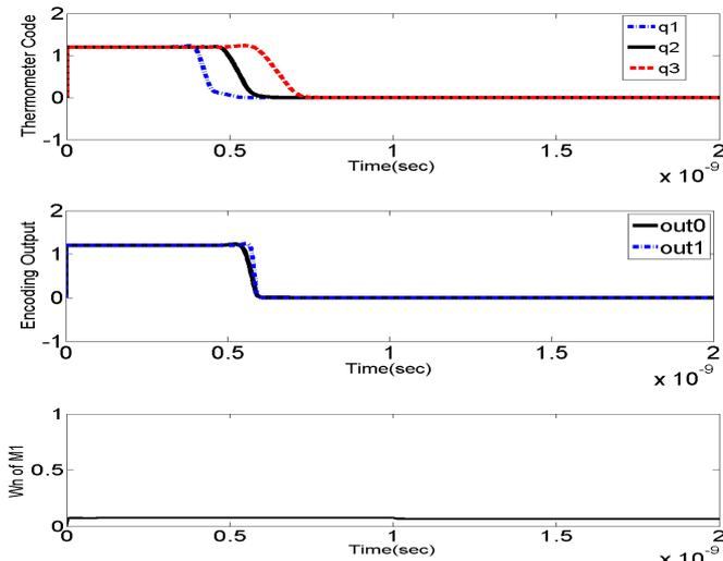
Figure 9. Reading state of M1 in case of 00.
