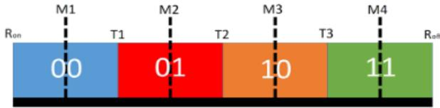
Figure 2. Multi-bit memristor storing 2-bits values [8].
