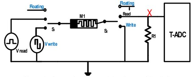
Figure 4. Connection between Memristor and T-ADC.
