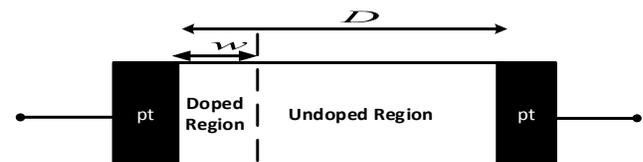
Figure 1. Memristor Device Structure.
