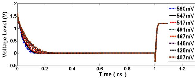
Figure 7. Output wave form of starved inverter at different input voltage in case of 3-bits.
