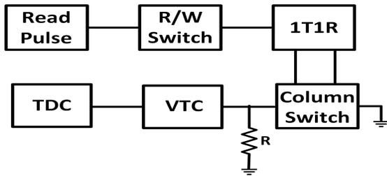
Figure 4. Proposed block diagram for reading operation.
