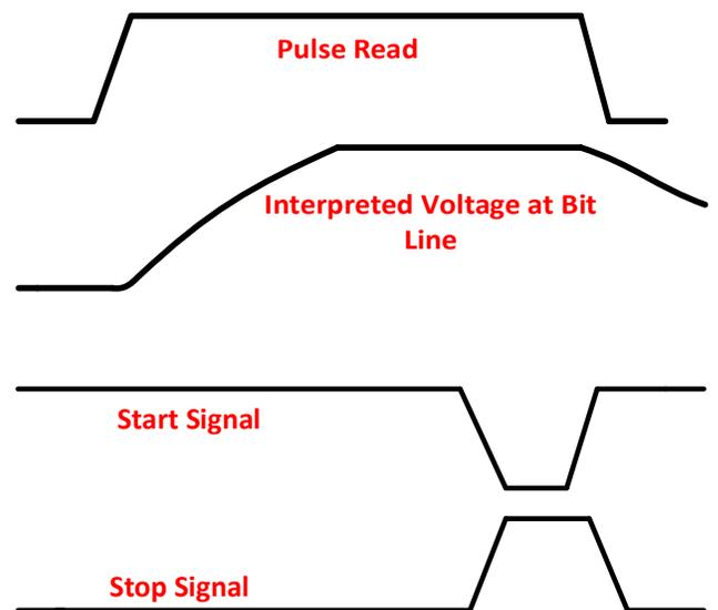
Figure 6. Timing diagram for the proposed circuit.
