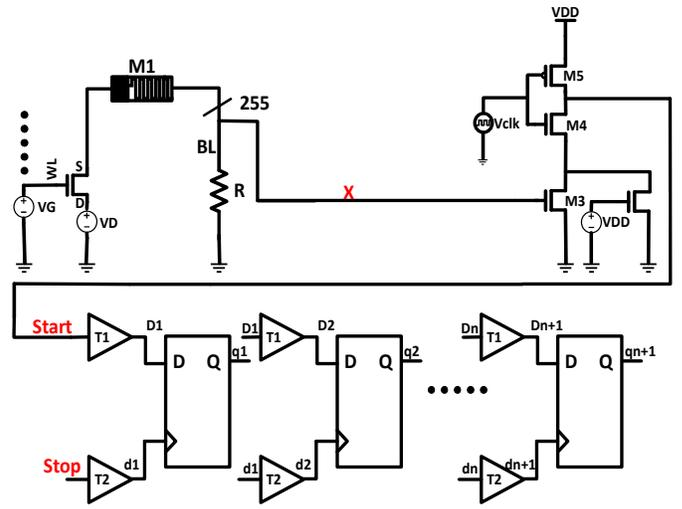
Figure 5. The simplified schematic of time to digital read path.
