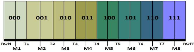
Figure 3. Memristor storing 3-bits value.
