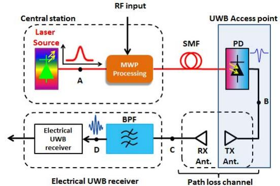
Fig. 1. Block diagram of a typical IR-UWBoF communication system. Red lines: optical paths. Black lines: electrical paths.
