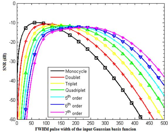
Fig. 2. Average SNR versus the FWHM pulse width of the Gaussian input basis function. Solid lines: theoretically obtained results. Markers: Results obtained by numerical integration techniques.
