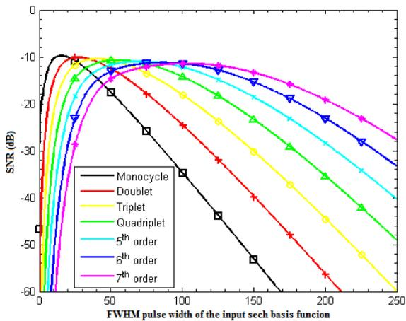
Fig. 3. Average SNR versus the FWHM pulse width of the sech input basis function. Solid lines: theoretically obtained results. Markers: Results obtained by numerical integration techniques.
