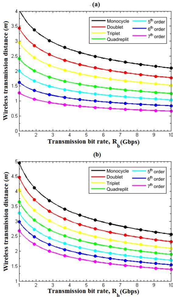
Fig. 3. Wireless transmission distance vs. the transmission bit rate with IR-UWB signalling using (a): Gaussian-input basis function and (b): sech input basis function at different values of  $m$
