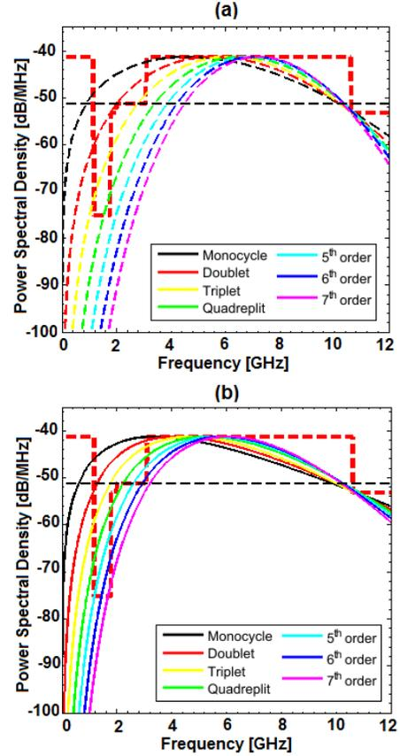
Fig. 2. Simulated electrical RF spectra of (a): Gaussian-based IR-UWB waveforms and (b): sech-based IR-UWB waveforms. Red dashed line: the FCC spectral mask. Black dashed line: the -51.3 dBm/MHz power spectral density limit to determine the -10 dB bandwidth.
