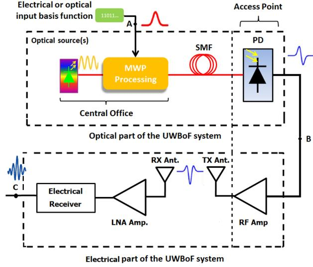
Fig. 1. Typical block diagram of an IR-UWBoF system with combined optical and wireless transmission. MWP: microwave photonic, SMF: single mode fiber, PD: photodetector, RF: radio frequency, Amp: amplifier, and LNA: low noise amplifier. Red lines: optical signal routes. Black lines: electrical signal routes.
