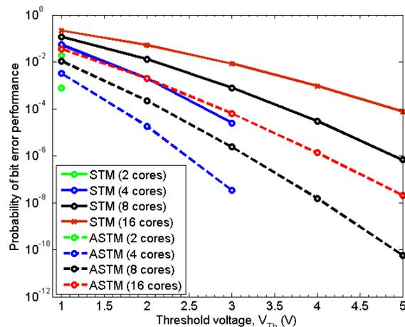
Fig. 5. Impact of threshold variation on the BER performance of OCC-based PNoC for cores operating in the synchronous and asynchronous transmission modes.
