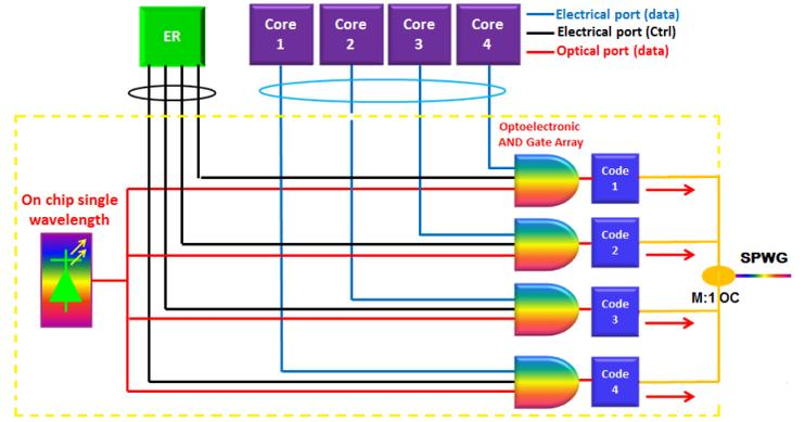
Fig. 2. Schematic diagram of the transmitter part of the proposed PNoC design. OC: optical coupler. By definition, an optoelectronic AND gate operates on electrical and optical logic inputs and generates only an optical logic output.
