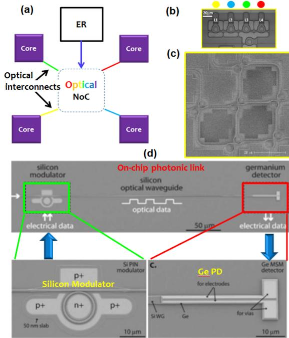
Fig. 1. Typical architecture and basic building blocks of PNoCs. (a): Block diagram of an electronic controlled optical routing network on chip. (b): four wavelength array of on-chip LD (from [7]). (c): an array of photonic switching elements (from [8]). (d): a typical on-chip photonic link, based on a single wavelength LD, a direct path silicon photonic waveguide and a Germanium-based photodetector (from [9]). ER: electronic router.
