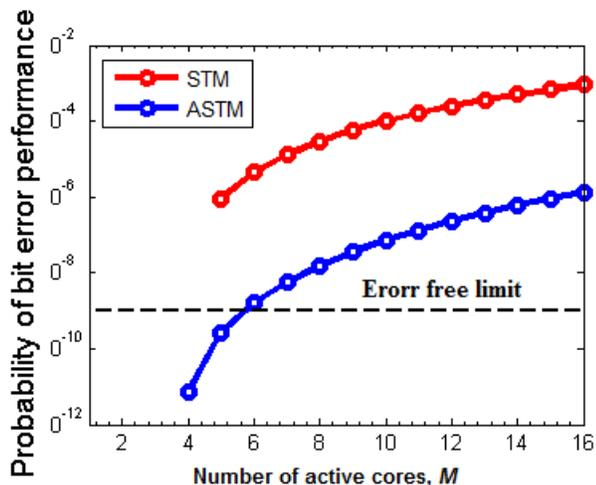
Fig. 4. BER performance versus the number of active cores,  $M$  sharing the PNoC. STM : synchronous transmission mode. ASTM : asynchronous transmission mode.
