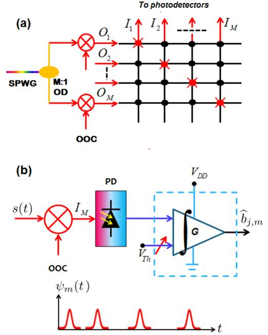
Fig. 3. Schematic diagram of the receiver part of the proposed PNoC design. (a): an  $M \times M$  passive photonic switching element array. Black dots: ON/OFF mode photonic switching elements. Red dots: only OFF mode photonic switching elements. (b): post photodetection processing at the receiver side. OD: optical divider. SPWG: silicon photonic waveguide.
