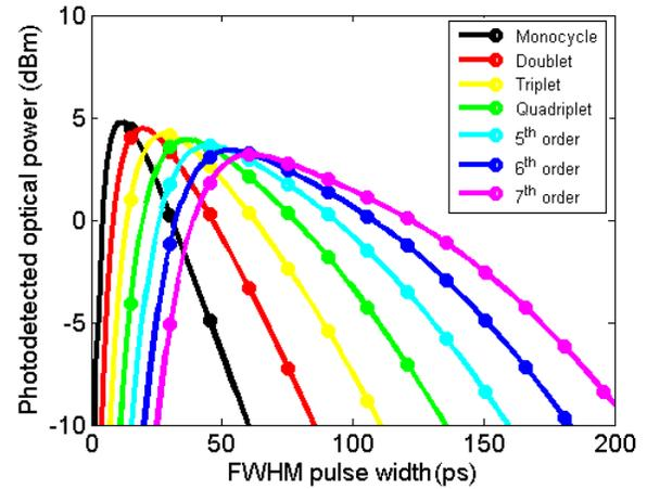
Fig. 4. Average photodetected optical power versus the FWHM pulse width of sech-based IR-UWB waveforms. Solid lines: theoretically obtained results. Markers: Results obtained by numerical integration techniques.
