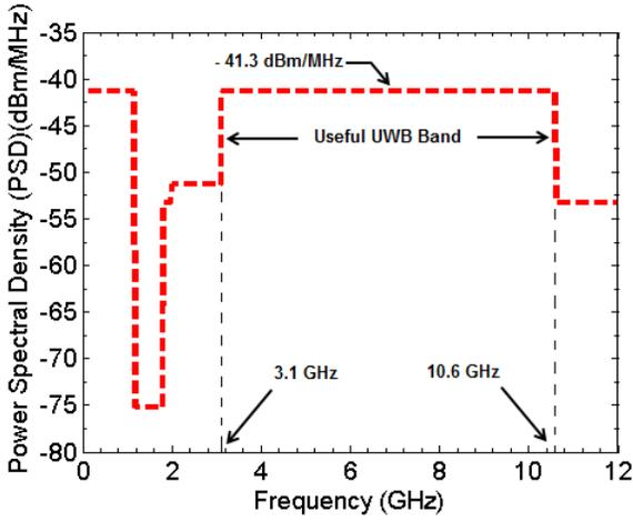
Fig. 2. The spectral constraints of the FCC mask.
