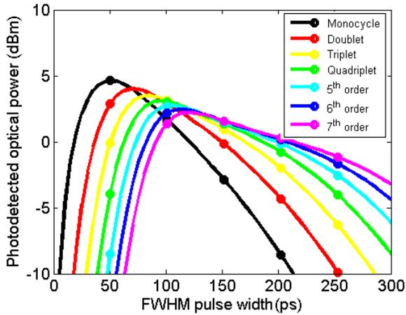
Fig. 3. Average photodetected optical power versus the FWHM pulse width of Gaussian-based IR-UWB waveforms. Solid lines: theoretically obtained results. Markers: Results obtained by numerical integration techniques.
