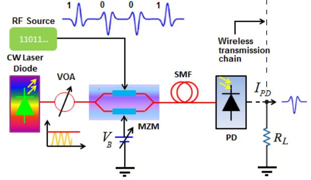
Fig. 1. Block diagram of a typical IR-UWB communication system. Red lines : optical paths. Black lines : electrical paths.
