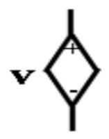
Voltage controlled voltage source (VCVS)
