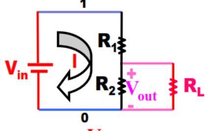
$$V_{out} = V_{AB} = I R_2 = \frac{V_{in}}{R_1 + R_2} R_2 = V_{in} \frac{R_2}{R_1 + R_2}$$
