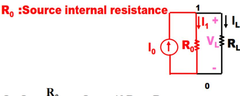
$$I_{L} = I_{0} \frac{R_{0}}{R_{L} + R_{0}} \approx I_{0}$$
