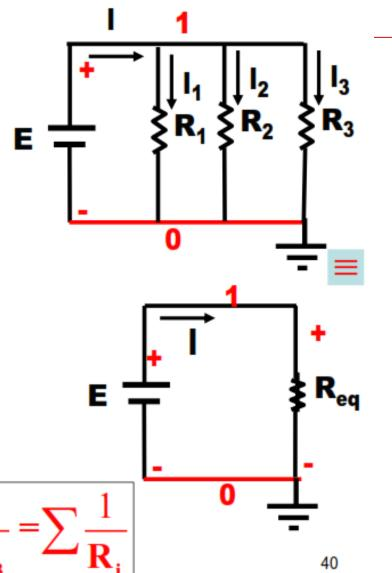
$$\overline{R_{eq}} = \overline{R_1} + \overline{R_2} + \overline{R_3} = \overline{R_i}$$
