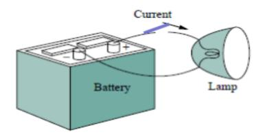
Three basic components: a battery, a lamp, switch and connecting wires.
