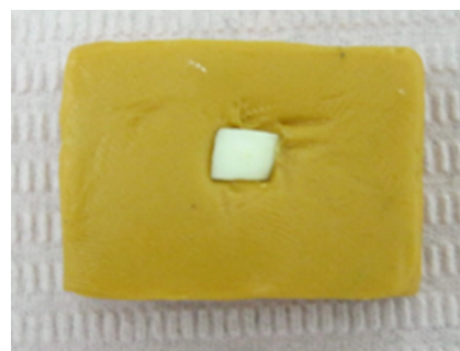
Figure 3. Dentin Slab Embedded in a Rubber Mold
