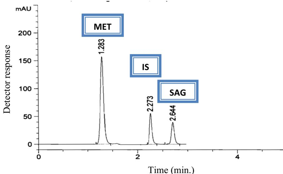
**Fig. 3.** HPLC chromatogram of a resolved mixture of MET (500 μg/mL,  $t_R = 1.283$ ), HZ (IS) (10 μg/mL,  $t_R = 2.273$ ) and SAG (2.5 μg/mL,  $t_R = 2.644$ ) using mobile phase of acetonitrile:phosphate buffer pH = 4.5 ± 0.1 (13:87, v/v) and Kinetex™ C<sub>18</sub> column – (4.6 × 150 mm), particle size (2.6 μm).
