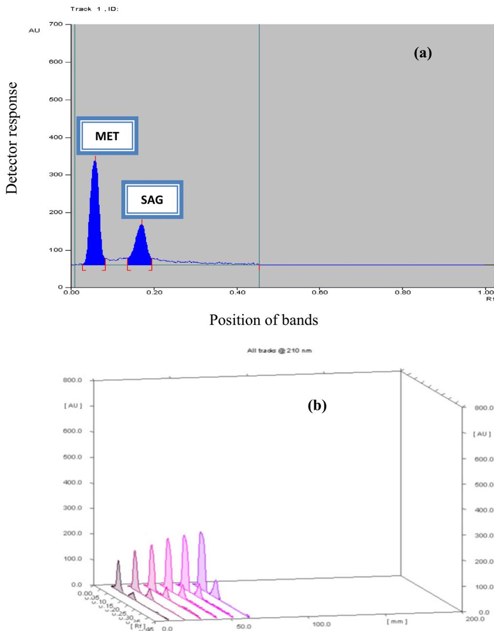
**Fig. 2.** (a) TLC chromatogram (2D) of a resolved mixture of MET (10  $\mu$ g/band,  $R_f$  = 0.06) and SAG (2  $\mu$ g/band,  $R_f$  = 0.17) (b) TLC chromatogram (3D) of mixtures of SAG and MET at 210 nm using chloroform:methanol:formic acid (80:20:0.3, by volume) as a developing system.
