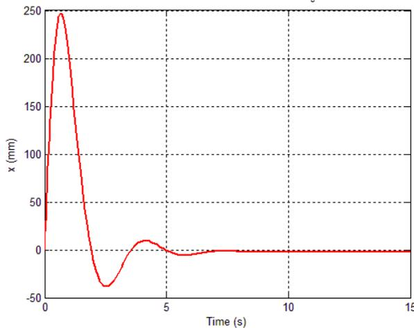
Fig.8 Dynamic response of the barrel assembly upon firing with  $\theta_0 = 20^\circ$ .
