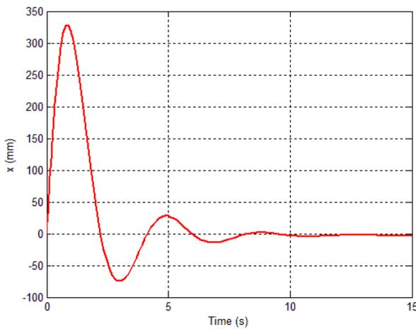
Fig.10 Dynamic response of the barrel assembly upon firing with  $\theta_0 = 40^\circ$ .
