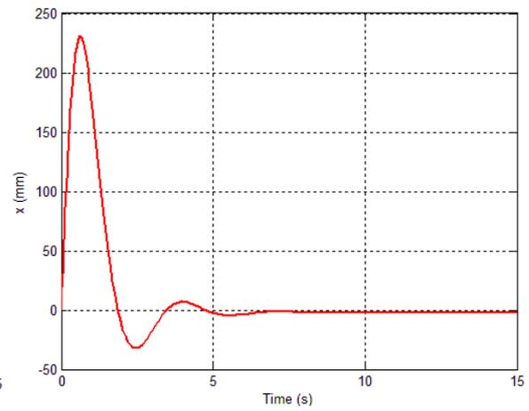
Fig.7 Dynamic response of the barrel assembly upon firing with  $\theta_0 = 10^\circ$ .
