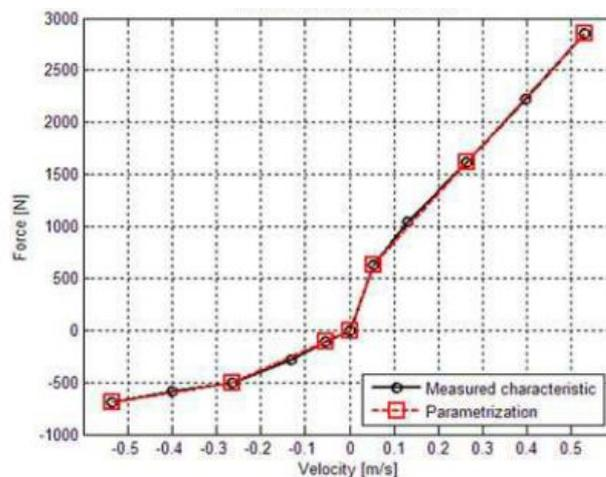
Fig.5 Typical damping characteristics of a hydraulic damper.
