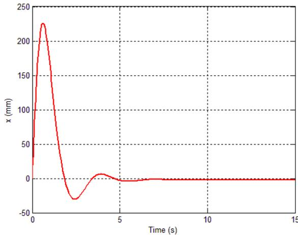
Fig.6 Dynamic response of the barrel assembly upon firing with  $\theta_0 = 0$ .
