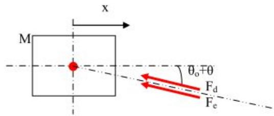
Fig.4 Free body diagram of the barrel assembly.
