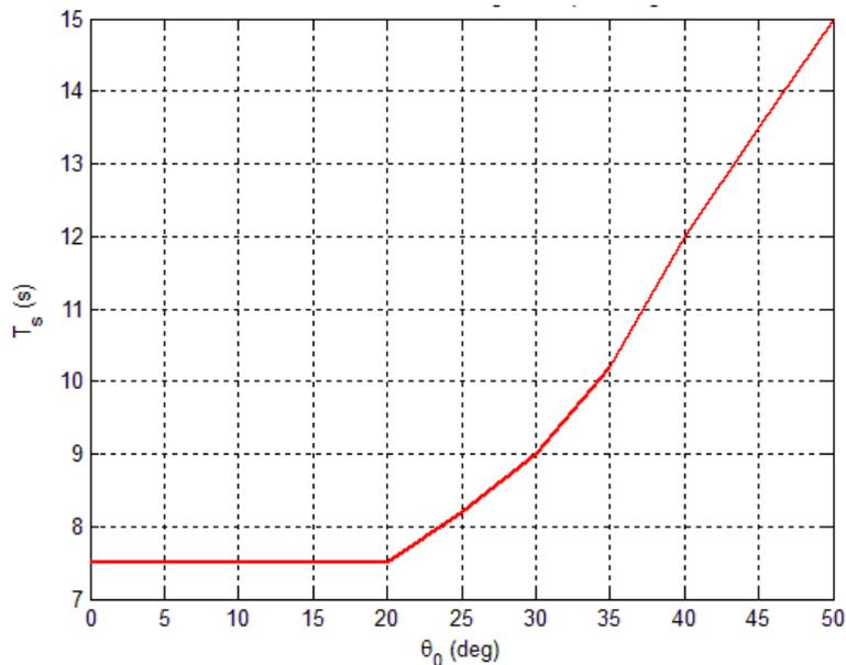
Fig.14. Settling time of the barrel assembly.
