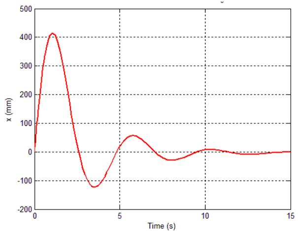
Fig.11 Dynamic response of the barrel assembly upon firing with  $\theta_0 = 50^\circ$ .
