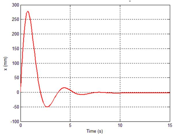
Fig.9 Dynamic response of the barrel assembly upon firing with  $\theta_0 = 30^\circ$ .
