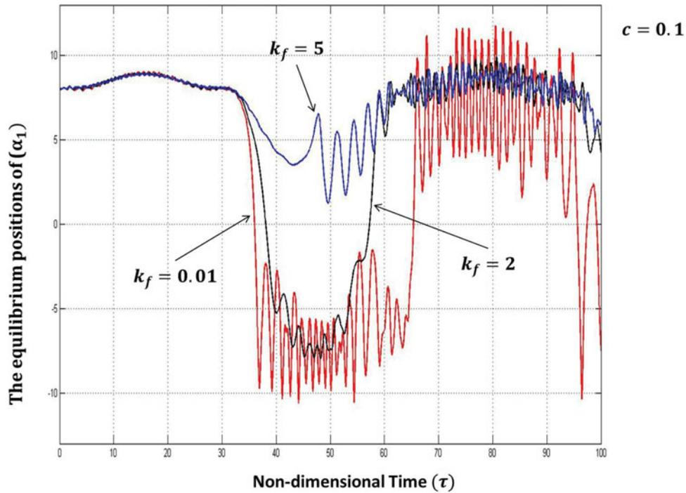
Figure 2. The dynamic response for an arch with  $h = 8$ ,  $Q = -40$  and  $c = 0.1$  for different fluids.
