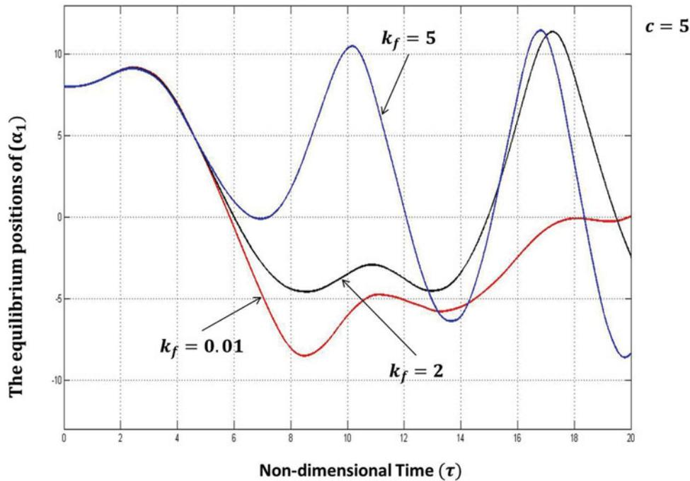
Figure 4. The dynamic response for an arch resting on different fluids with  $h = 8$ ,  $Q = -40$  and  $c = 5$ .
