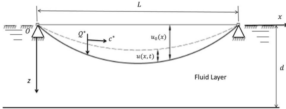
Figure 1. Schematic diagram of a shallow arch resting on a finite fluid layer under a moving point load.
