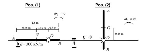
Assume the initial horizontal position of the rod is denoted by pos. (1) and vertical position is denoted by pos. (2).
