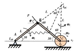
Using the instantaneous center method, the hinge A is the I.C. of the rod AB, then using I.C. of AB, the direction of  $\underline{v}_B$  will be normal to AB. Draw perpendicular lines to the directions of the  $\underline{v}_B$  and  $\underline{v}_C$  which moves on a horizontal line passing through A, then one can obtain the I.C. of the rod BC. Since the disc rolls, then the point D is the I.C. of the disc.
