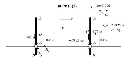
External Forces System (E.F.S) Inertia Forces System (I.F.S)
