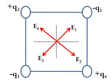
$E_{1x} = E_1 \cos 45 = 102 \times 10^3 \text{ N/C}$   $E_{2x} = E_2 \cos 45 = 51 \times 10^3 \text{ N/C}$   $E_{3x} = -E_3 \cos 45 = -51 \times 10^3 \text{ N/C}$  $E_{4x} = -E_4 \cos 45 = -102 \times 10^3 \text{ N/C}$
