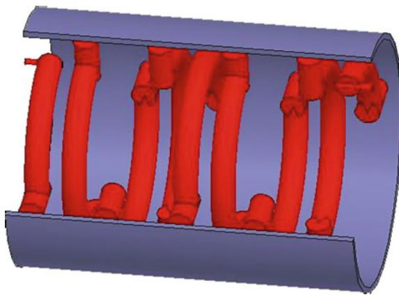
**a** 8-Cells Backward Wave Waveguide (inside view).
