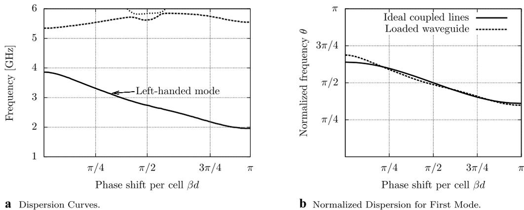
**Fig. 3** (a) Dispersion curves of the metaguide obtained using FEM, where the *dotted lines* are for higher modes, and (b) normalized dispersion of LH mode of subfigure (a) compared to that obtained from circuit
