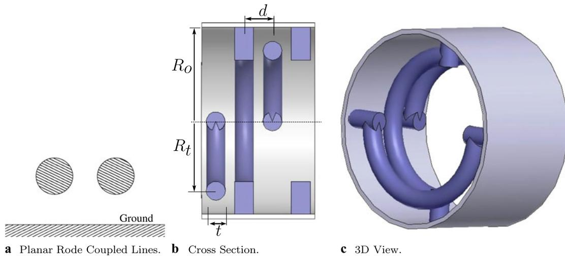
**Fig. 2** (a) Cross section of planar coupled circular rods, (b) cross section of cylindrical waveguide loaded with rode coupled lines, and (c) 3D view of subfigure (b)
