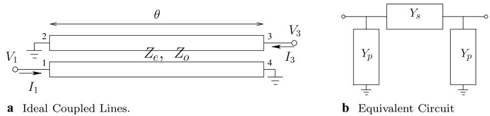
of the coupled lines of physical length  $L$ . The considered coupled line has no dielectric filling, hence its propagation factor  $k = \omega/c$ , where  $c$  is the speed of light in vacuum. The parameters  $Y_o$  and  $Y_e$ , are the odd and even admittance, respectively. The proposed unit cell can be modeled by the  $\Pi$  network shown in Fig. 1(b). In this equivalent circuit the series  $Y_s$  and parallel  $Y_p$  are given in terms of the elements of the admittance matrix (1) by [9]
