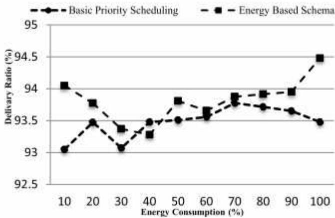
Fig. 4 Network Energy consumption vs. Packet Delivery Ratio
