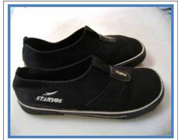
Figure 3. A pair of thin flexible-soled shoes with stretchable body to fit adequately to the patients' feet. Thin flexible-soled shoes were tested so that the loads on the force plate would not be dampened by thick inflexible ones. 52
