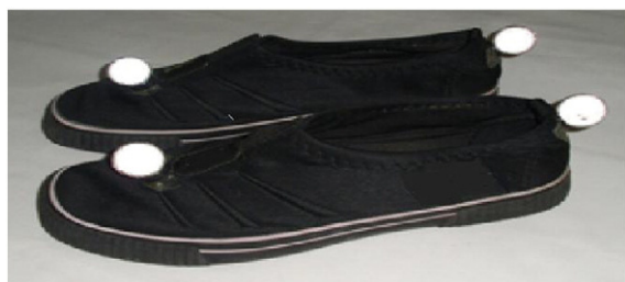
Fig. 3. Flexible shoes with the reflective markers place on top.
