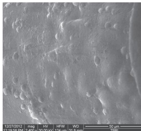
Scanning electron micrograph of an endotracheal tube at higher magnification showing (grade 1) bacterial biofilm (x2400) with scattered large cocci. The duration of intubation was 2 days.
