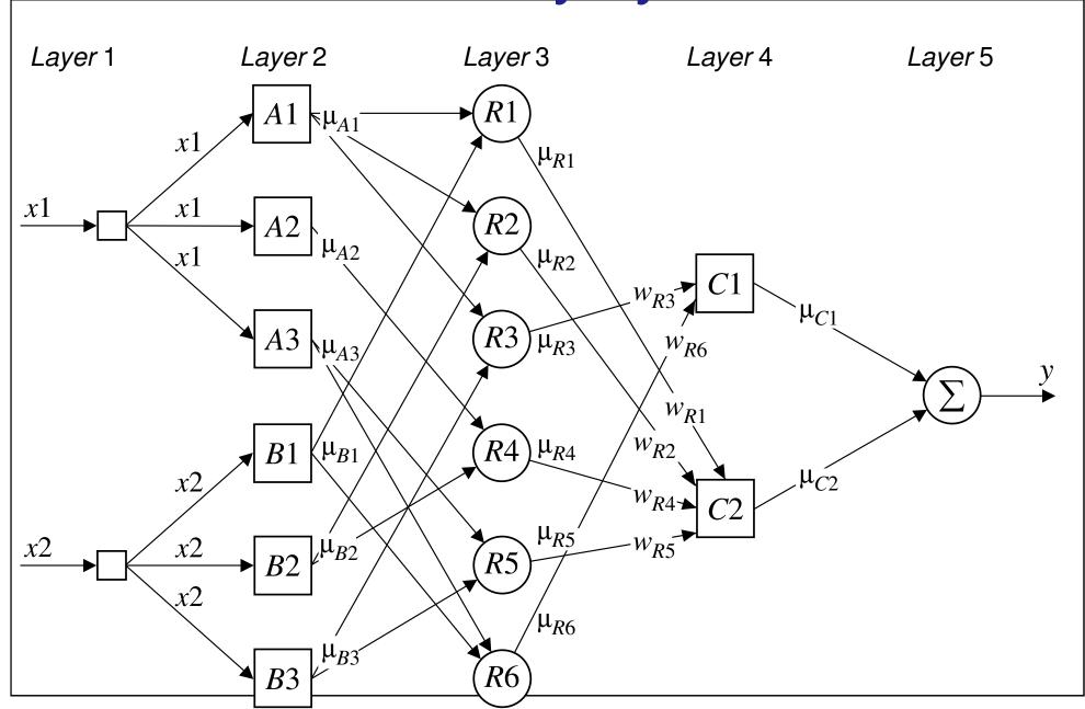
Each layer in the neuro-fuzzy system is associated with a particular step in the fuzzy inference process.
