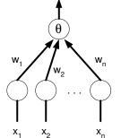
if  $\Sigma W_i X_i >= \mathbf{0}$ , output = 1 if  $\Sigma W_i X_i < \mathbf{0}$ , output = 0
