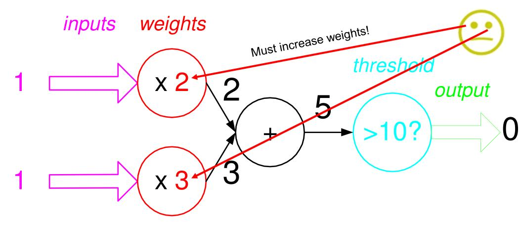
If both inputs are 1, output should be 1.
