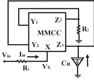
Fig. 2. The proposed current-controlled memristor emulator.
