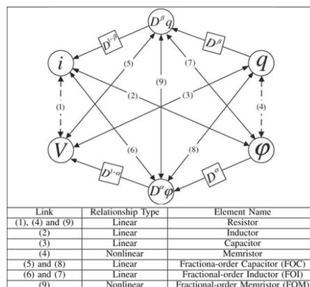
Fig. 1. The relation between fractional-order elements and memelements.
