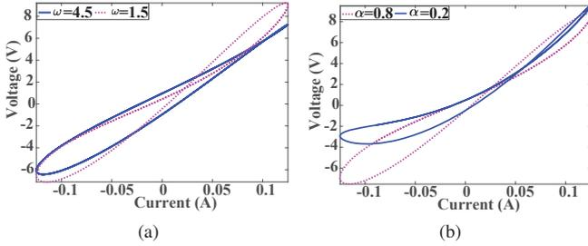
Fig. 7. Numerical simulations of series fractional memristor and FOI at different (a)  $\omega$  at  $\alpha = \beta = 0.7$ , (b)  $\alpha$  when  $\beta = 0.8$  and  $\omega = 1.5$ .
