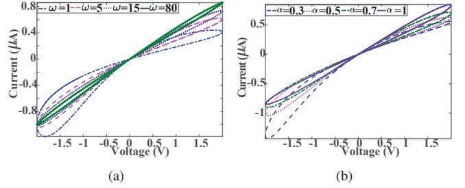
Fig. 3. Numerical simulations of memductance for  $a = 9 \times 10^{-5}$  at different (a) frequencies when  $\alpha = 0.7$ , and (b)  $\alpha$  when  $f=0.16\text{Hz}$
