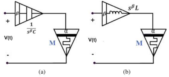
Fig. 4. Series fractional-order memristor with (a) FOC, and (b) FOI.
