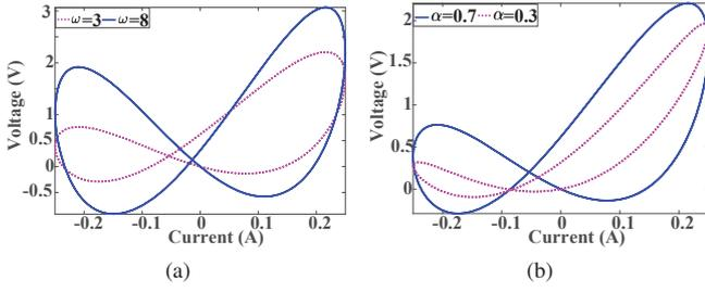
Fig. 6. Numerical simulations of fractional-order inverse memristor connected in series with FOI at different (a)  $\omega$  at  $\alpha = \beta = 0.7$ , and (b)  $\alpha$  when  $\beta = 0.8$  and  $\omega = 3$
