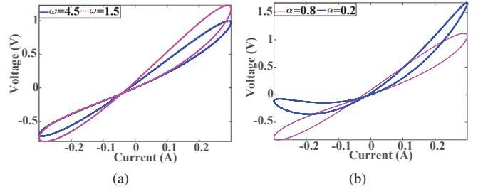
Fig. 5. Numerical simulations of fractional-order memristor connected in series with FOC at different (a)  $\omega$  when  $\alpha = \beta = 0.7$  (b)  $\alpha$  when  $\beta = 0.8$  at  $\omega = 4.5$ .
