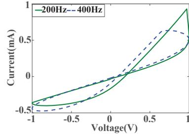
Fig. 10. The simulation results of the series connection of the fractional-order memristor and FOI at different frequencies.
