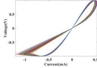
Fig. 9. The Monte Carlo results for the hysteresis loop of the memristor in the I-V plane at  $\alpha = 0.8$ .
