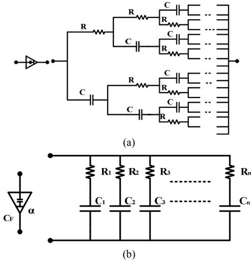
Fig.1. Approximation the capacitor with (a) order 0.5, and (b) general order
