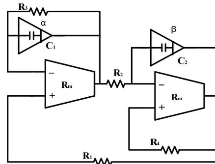
Fig.3. OTRA based oscillator
