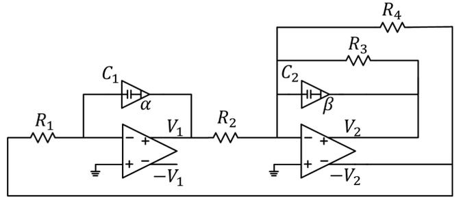
Fig.2: Soliman's four phase oscillator
