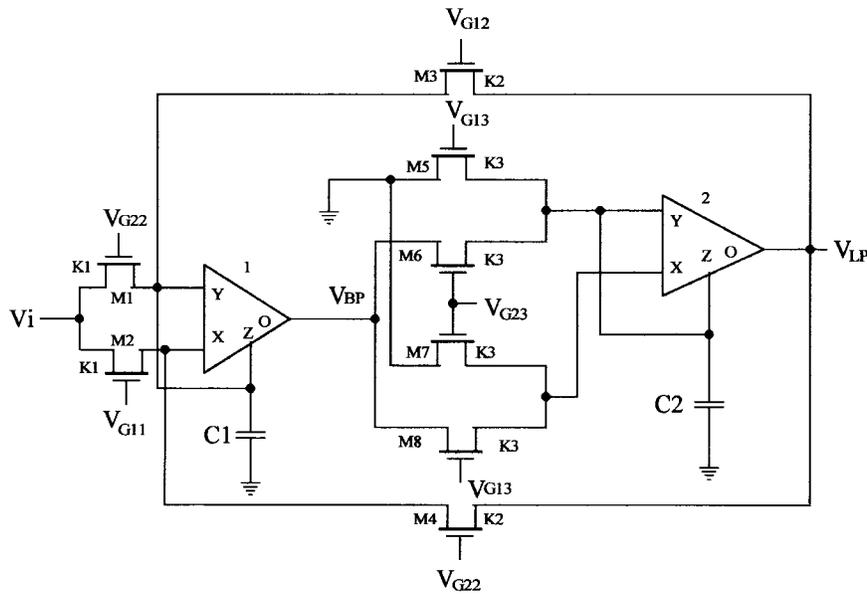
Fig. 2. The proposed MOS-C CFOA bandpass-low-pass filter.
