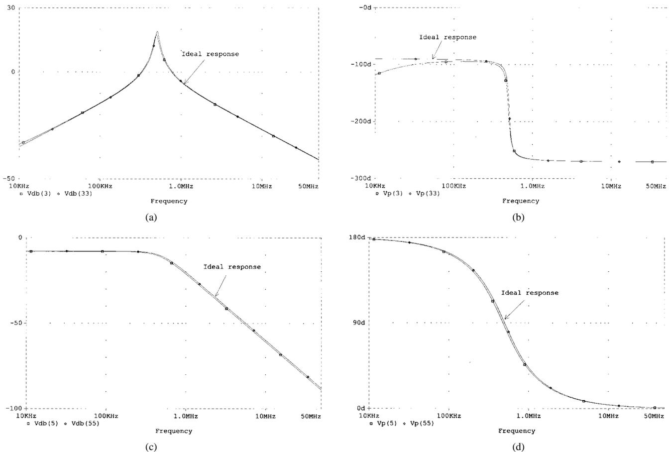
Fig. 3. (a) The magnitude response of the bandpass filter. (b) The phase response of the bandpass filter. (c) The magnitude response of the low-pass filter. (d) The phase response of the low-pass filter.
