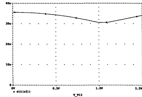
Fig. 9: The transconductance  $G_m$  of the proposed linearized long tail differential pair CMOS transconductor versus differential input voltage  $V_1$
