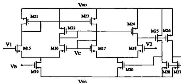
Fig. 5-b: The circuit schematic of the low voltage CMC
