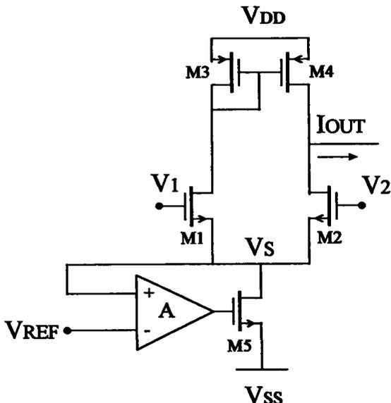
Fig. 2: The linearised long tail differential pair CMOS transconductor using an high gain amplifier
