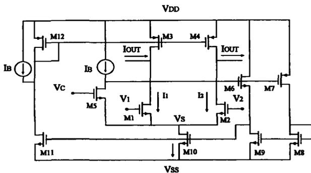
Fig. 4-a: The circuit schematic of the LDP
