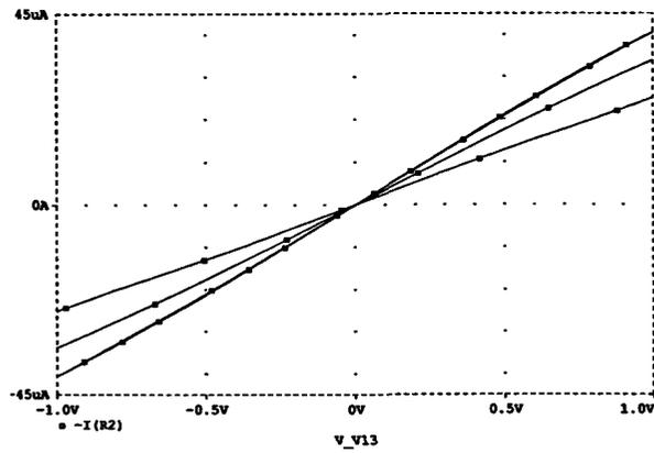
Fig. 7: The I-V characteristics of the proposed linearized long tail differential pair CMOS transconductor
