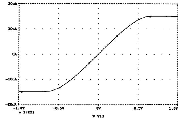
Fig. 6: The I-V characteristics of the ordinary long tail differential pair CMOS transconductor
