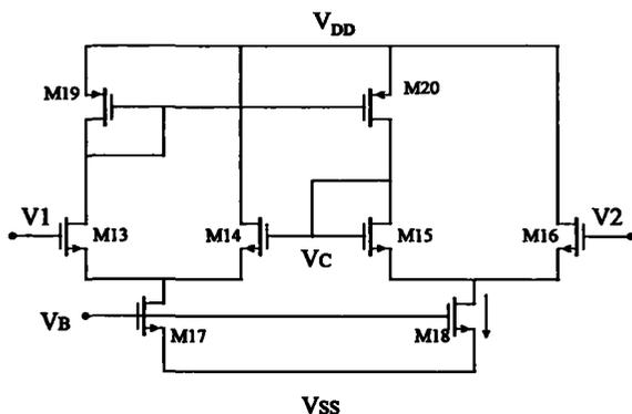
Fig. 4-b: The circuit schematic of the CMC
