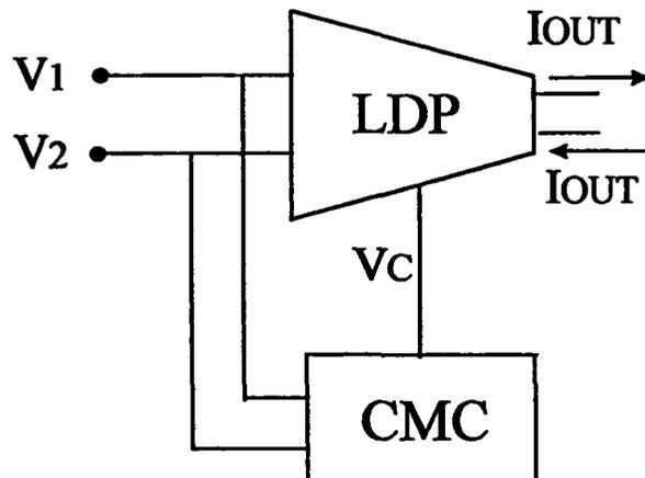
Fig. 3-c: The complete BOTA obtained by interconnecting the LDP and the CMC
