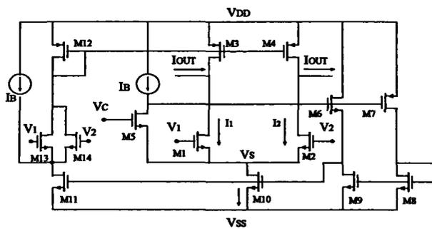
Fig. 5-a: The circuit schematic of the low voltage LDP
