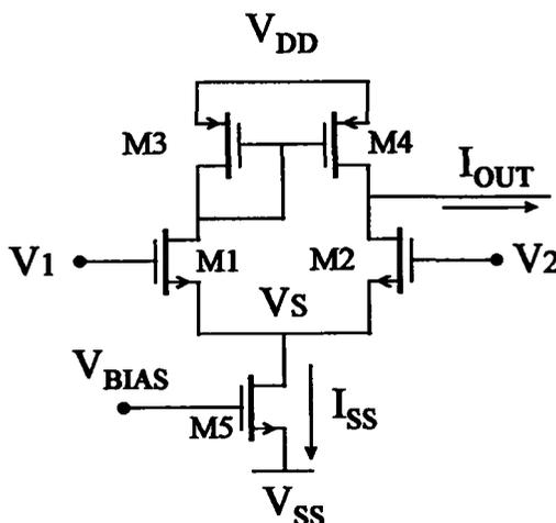
Fig. 1: The ordinary long tail differential pair CMOS transconductor
