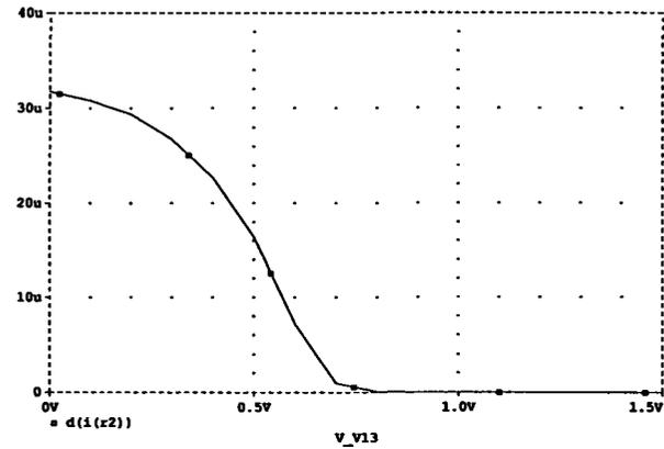
Fig. 8: The transconductance  $G_m$  of the ordinary long tail differential pair CMOS transconductor versus differential input voltage  $V_1$
