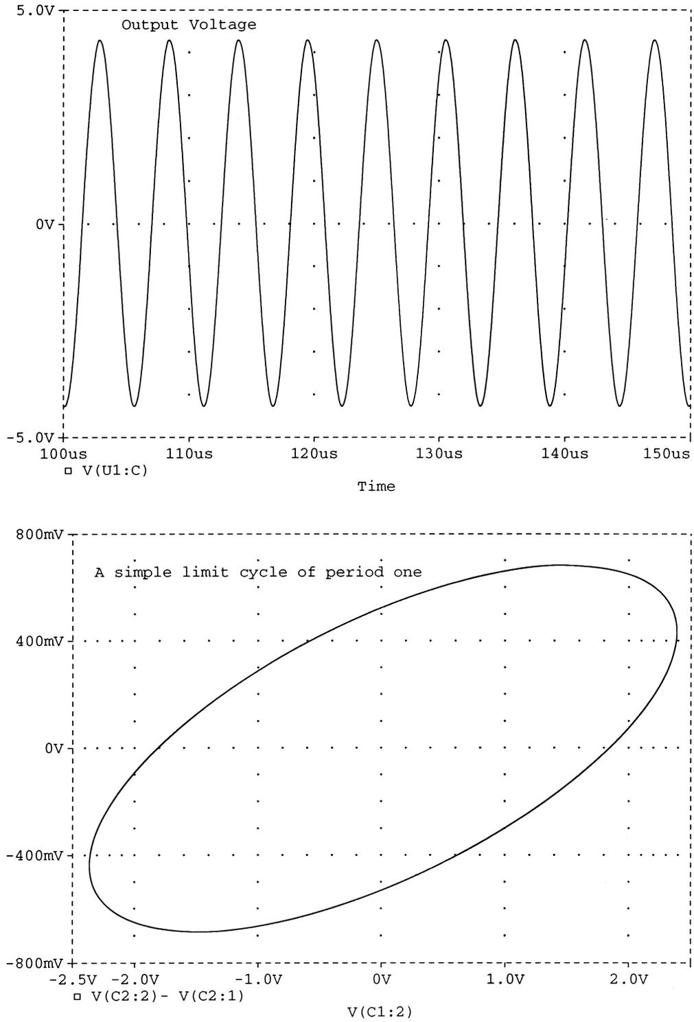
Fig. 2. (a) The output voltage waveform for the oscillator circuit of Fig. 1. (b)  $V_{C2}$  versus  $V_{C1}$  for the oscillator circuit of Fig. 1.
