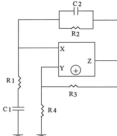
Fig. 1. A voltage mode oscillator derived from the well-known bandpass circuit [12].
