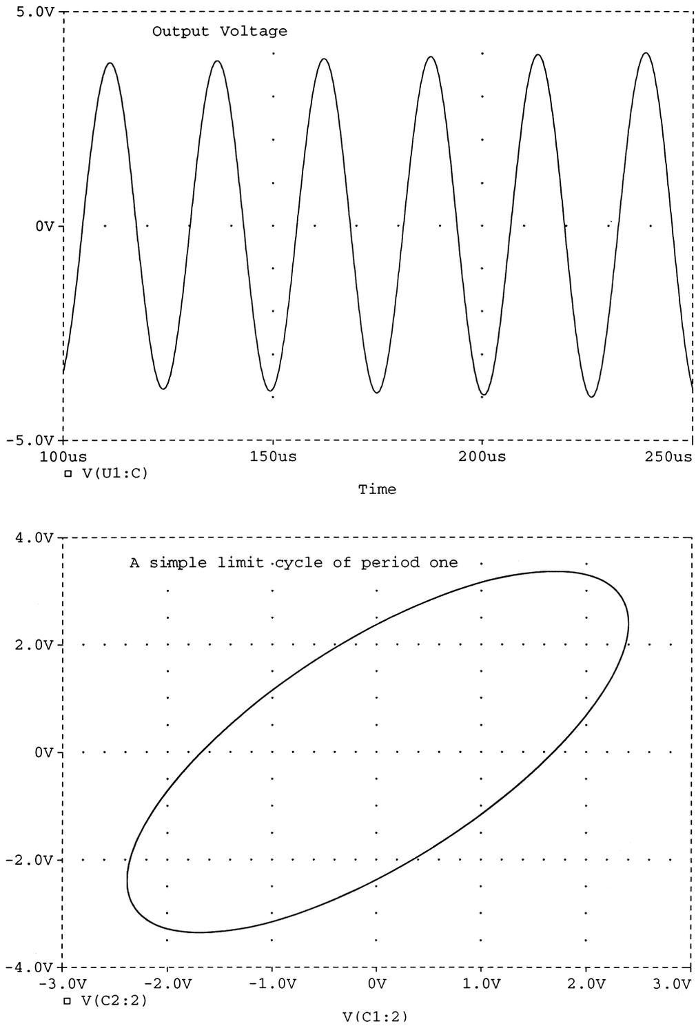
Fig. 4. (a) The output voltage waveform for the oscillator circuit of Fig. 3(b). (b)  $V_{C2}$  versus  $V_{C1}$  for the oscillator circuit of Fig. 3(b).
