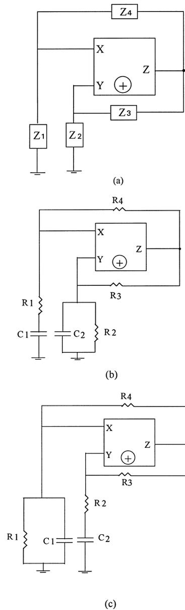
Fig. 3. (a) A generalized voltage mode oscillator using a single CCII based on the circuit of Fig. 1. (b) The new grounded capacitor voltage mode oscillator. (c) The unstable grounded capacitor circuit.
