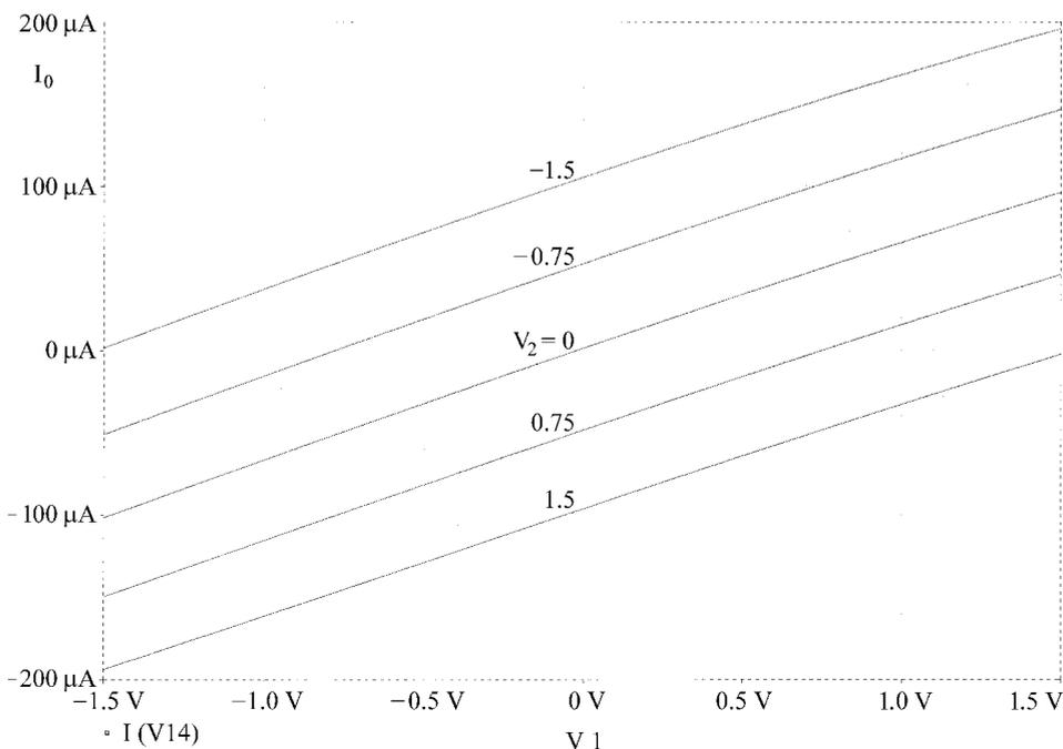
Figure 4. The output current of the BOTA.
