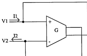
Figure 7. The BOTA-based floating resistor.
