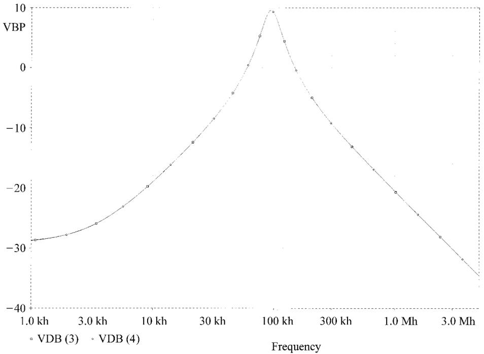
Figure 14. The magnitude response of the bandpass filter outputs.
