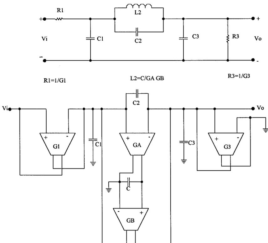
Figure 17. A third-order LCR filter and the corresponding active BOTAs-C realization.
