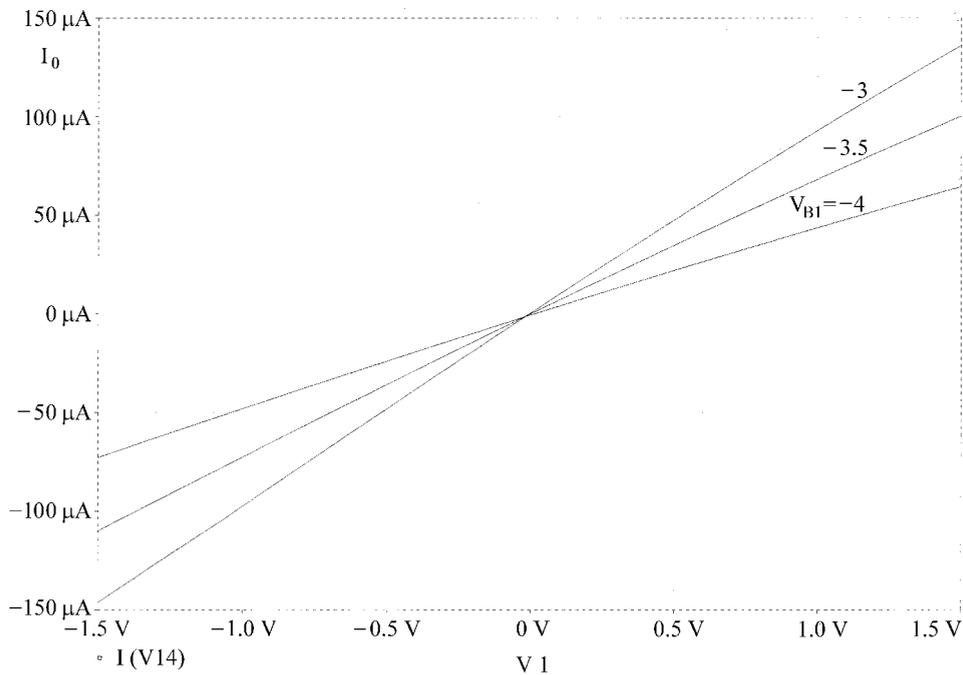
Figure 5. The output current of the BOTA with  $V_{B1}$  as a control parameter.
