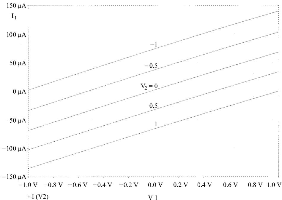
Figure 8. The  $I - V$  characteristics of the floating resistor.
