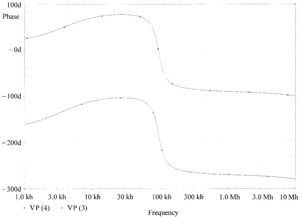
Figure 15. The phase response of the bandpass filter outputs.
