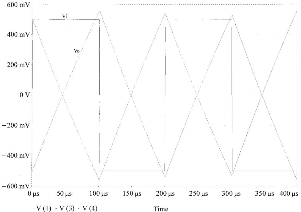
Figure 10. The input and the balanced outputs of the BOTA integrator.
