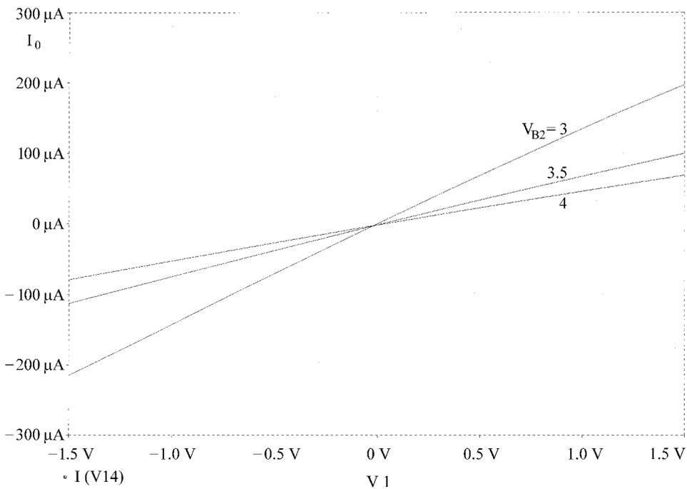
Figure 6. The output current of the BOTA with  $V_{B2}$  as a control parameter.
