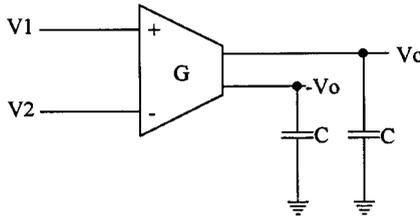
Figure 9. The BOTA-based balanced output differential integrator.
