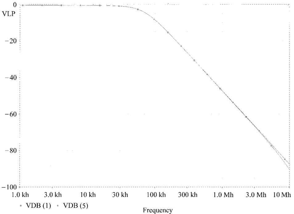
Figure 12. The magnitude response of the lowpass filter outputs.
