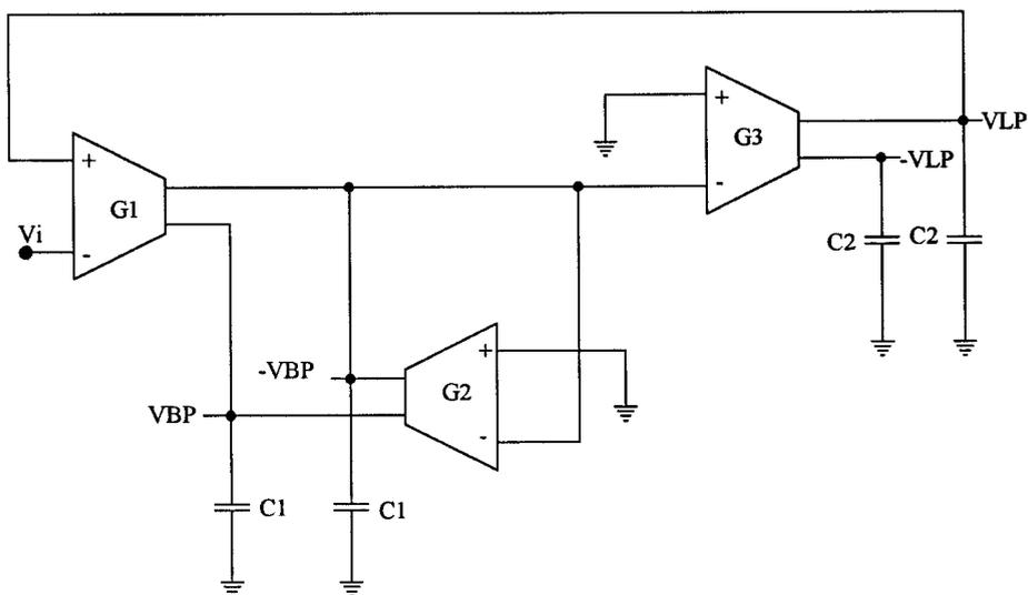
Figure 11. The BOTA-based balanced output bandpass–lowpass active filter.
