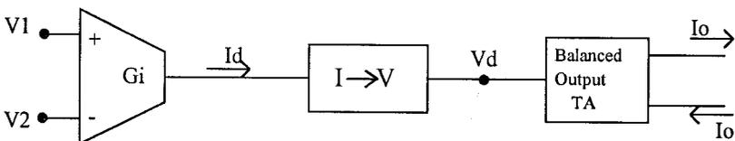
Figure 2. The proposed block diagram of the BOTA.
