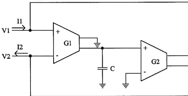
Figure 16. The BOTAs-based floating inductor circuit.
