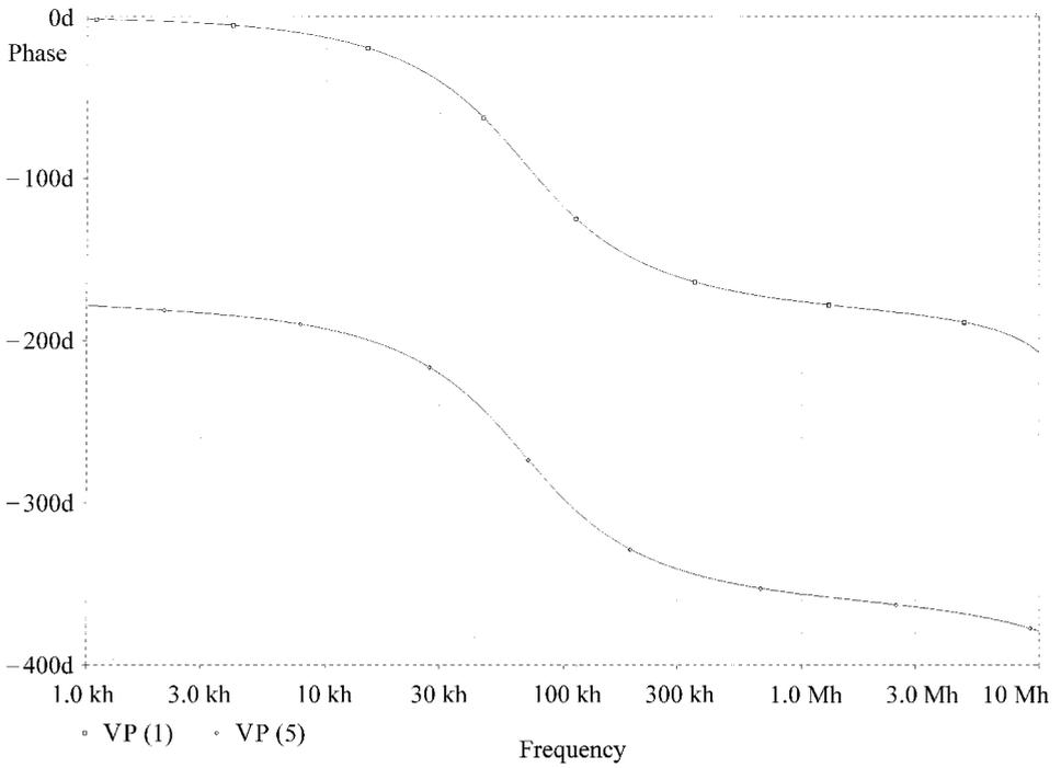
Figure 13. The phase response of the lowpass filter outputs.
