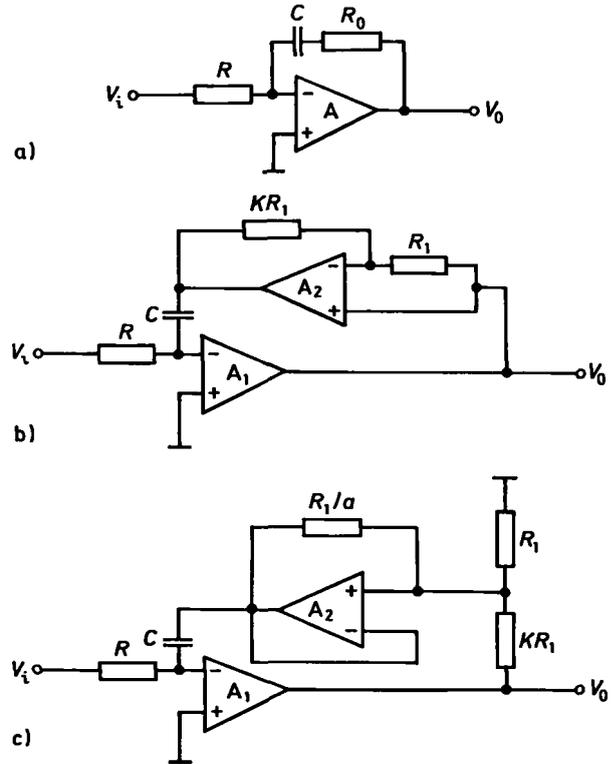
Fig. 2: Variable phase inverting integrators (see also table 1)
