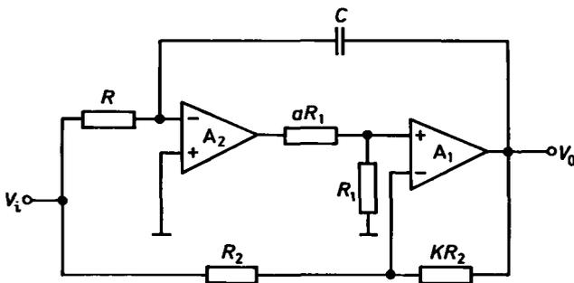
Fig. 1: Novel variable phase inverting integrator
