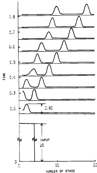
Fig. 3. Formation of solitary waves under the initial condition of rectangular input pulse.
