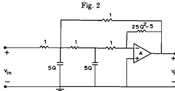
Sallen-Key negative feedback low-pass filter. Circuit components are given for  $\omega_0 = 1$ .
