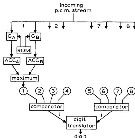
Fig. 1 Functional diagram of the digital multifrequency-tone detector
