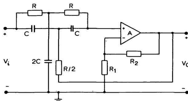
Fig. 1 Well known configuration for realising a low-selectivity notch filter
