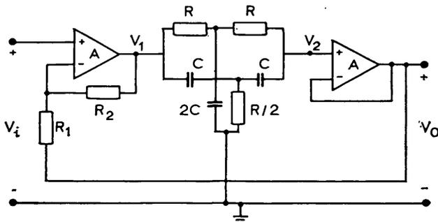
Fig. 2 New configuration for realising a medium-selectivity notch filter
