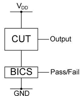
Fig. 4 Block diagram of BICS testing
