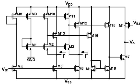
Fig. 18 CMOS realization of the OTRA under test [22]
