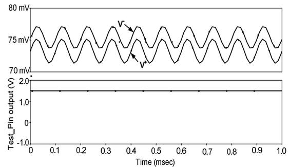
Fig. 21 The terminal voltages of OTRA along with the output of the BIS in case of open drain at transistor M8
