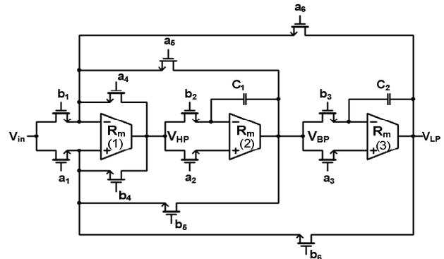
Fig. 23 The OTRA-based KHN biquad circuit used as CUT [22]
