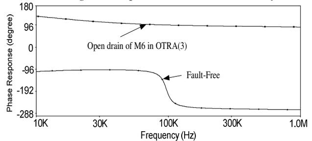
(b) the BP phase response of the fault-free and faulty filter
