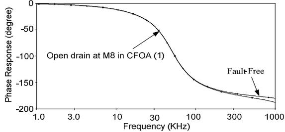
(b) The LP phase response of the fault-free and faulty filter
