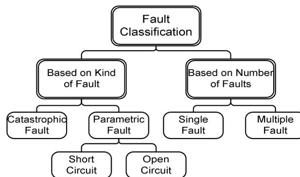
**Fig. 1 The Fault Classification**
