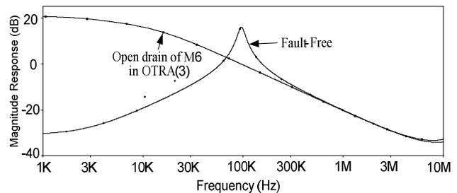
(a) the BP magnitude response of the fault-free and faulty filter
