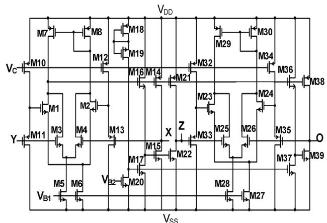
Fig. 7 CMOS realization of the tested CFOA[21]
