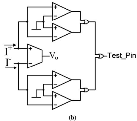
Fig. 17 (a) Structure of the proposed BIS, (b) Structure of the testable OTRA
