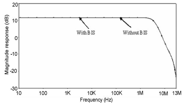
Fig. 11 The magnitude response of the CFOA-based amplifier with and without BIS
