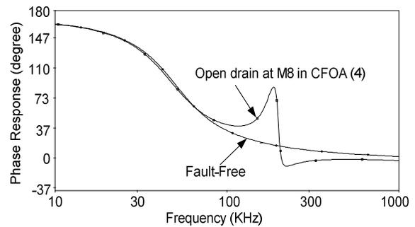
(b) The HP phase response of the fault-free and faulty filter and
