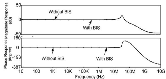
Fig. 22 The magnitude and phase response of the OTRA-based VCVS with and without connecting the BIS
