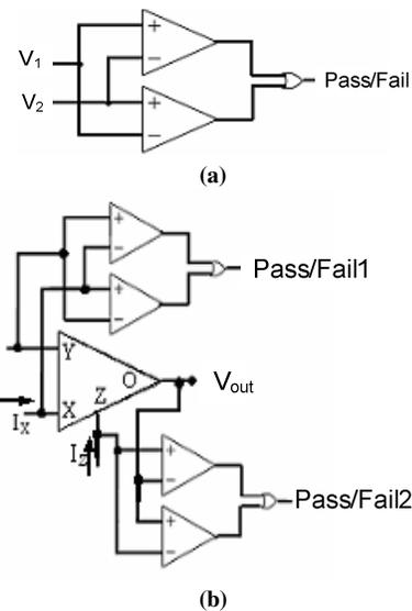
Fig. 6 (a) Structure of the proposed BIS, (b) Structure of the testable CFOA
