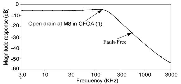
(a) The LP magnitude response of the fault-free and faulty filter
