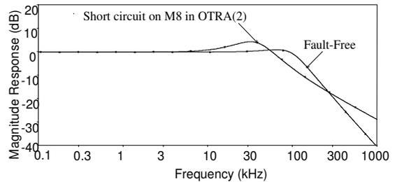
(a) the LP magnitude response of the fault-free and faulty filter
