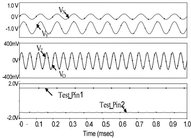
Fig. 8 The terminal voltages for the tested CFOA along with Test\_Pin1 and 2 in case of M12 is shorted.
