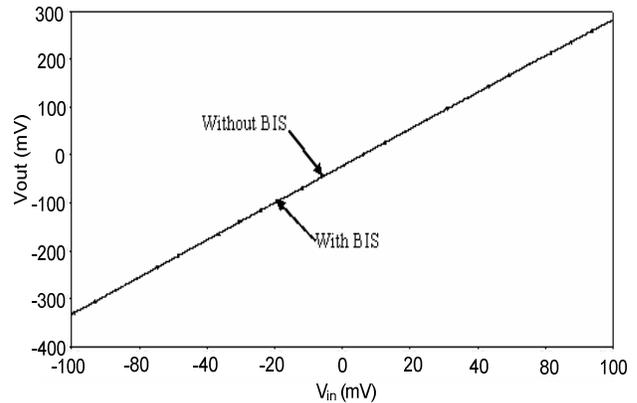
Fig. 10 CFOA-based amplifier output voltage with and without BIS
