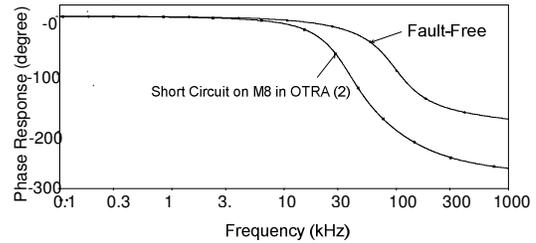
(b) the LP phase response of the fault-free and faulty filter
