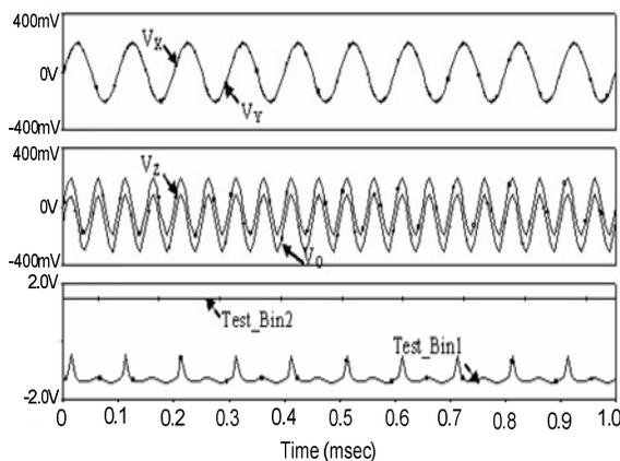
Fig. 9 The terminal voltages of the tested CFOA along with Test\_Pin 1 and 2 in case of open drain fault at M32
