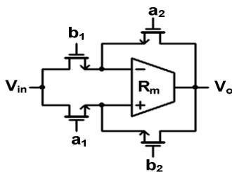
Fig. 19 The OTRA-based VCVS used as CUT [22]
