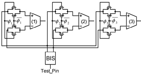
Fig. 24 The configuration of connecting OTRAs in the KHN filter example to the BIS
