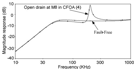
(a) The HP magnitude response of the fault-free and faulty filter,
