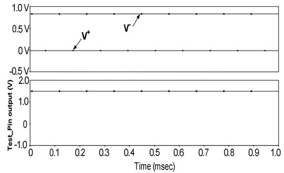
Fig. 20 The terminal voltages of OTRA along with the output of the BIS in case of short circuit on transistor M2
