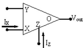
Fig. 5 Current Feedback Op-Amp symbol
