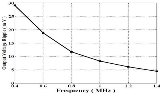
Figure 11. Output voltage ripple versus frequency (six-stage,  $V_{DD}=0.3V$ ,  $I_{out}=1\mu A$ ,  $C_{load}=25pF$ )
