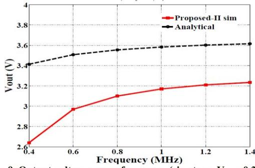
Figure 9. Output voltage versus frequency (six-stage,  $V_{DD}=0.3V$ ,  $I_{out}=1\mu A$ )
