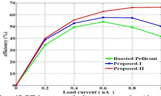
Figure 15. Efficiency versus load current comparison (six-stage,  $V_{DD}=0.3V$ ,  $f=1MHz$ )
