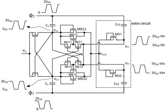
Figure 7. Proposed output stage of modified Pelliconi pump
