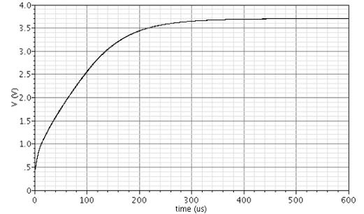
Figure 8. Initial transient (six-stage,  $V_{DD}=0.3V$ ,  $f=1\text{MHz}$ ,  $C_{load}=25\text{pF}$ ,  $I_{out}=0$ )
