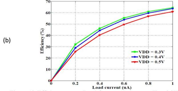
Figure 13. Efficiency versus Load Current a) six-stage,  $V_{DD}=0.3V$  b) Three-Stage,  $f=1MHz$
