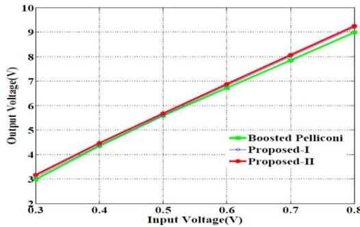
Figure 16. Gain comparison (six-stage,  $I_{out}=1\mu A$ ,  $f=1MHz$ )
