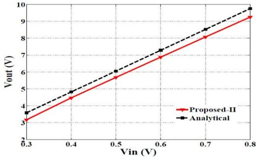
Figure 10. Output voltage versus input voltage (six-stage,  $I_{out}=1\mu A$ ,  $f=1MHz$ )
