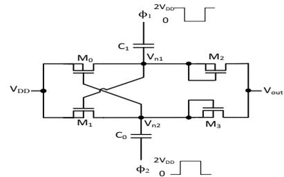
Figure 6. Output stage of modified Pelliconi CP
