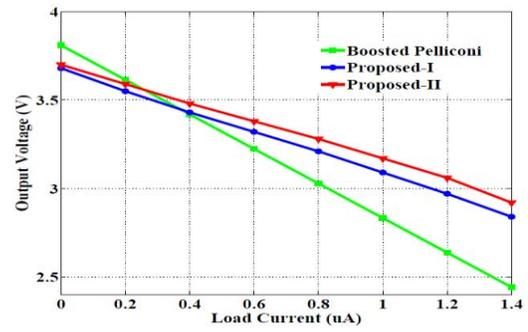
Figure 17. Output voltage versus output current comparison (six-stage,  $V_{DD}=0.3V$ ,  $f=1MHz$ )
