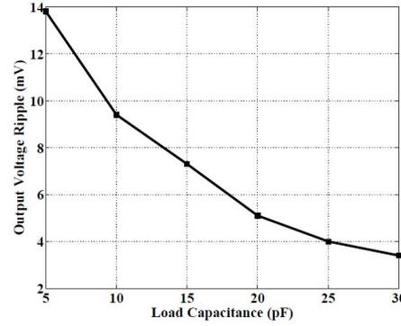
Figure 12. Output voltage ripple versus load capacitance (six-stage,  $V_{DD}=0.3V$ ,  $I_{out}=0.5\mu A$ ,  $f=1MHz$ )
