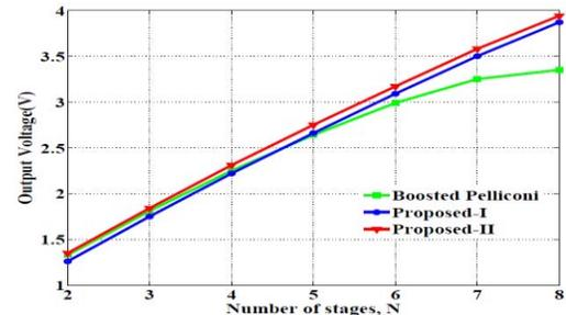
Figure 18. Output voltage versus number of stages comparison ( $V_{DD}=0.3V$ ,  $f=1MHz$ ,  $I_{out}=1\mu A$ )
