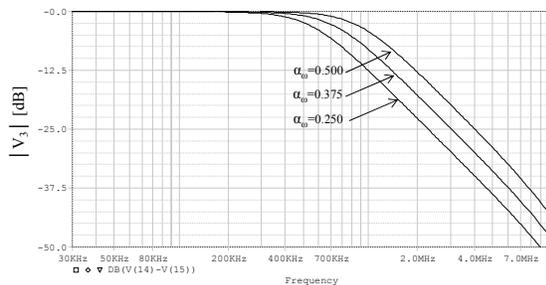
Fig. 8: Magnitude Response of the Differential Voltage Lowpass Output.
