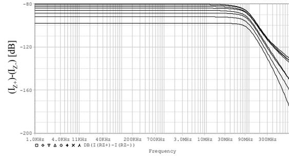
Fig. 5: AC Response of the Z-Terminals Current of the DCFDCC.
