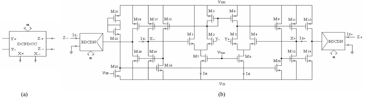
Fig. 3: (a) Symbol of the DCFDCC (b) CMOS Realization of the DCFDCC
