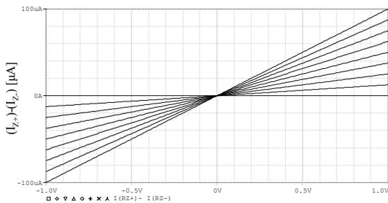
Fig. 4: DC Response of the Z-Terminals Current of the DCFDCC.
