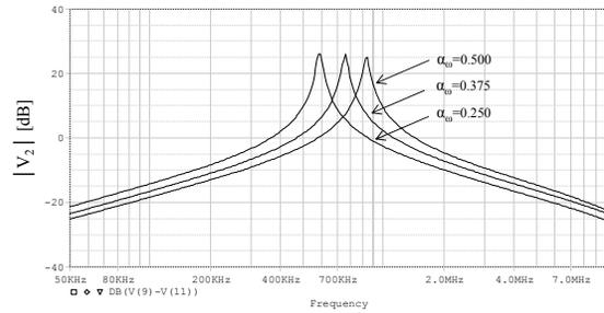
Fig. 9: Magnitude Response of the Differential Voltage Bandpass Output.
