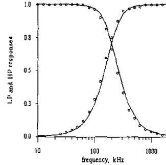
Fig. 3. The measured Lowpass and the Highpass Butterworth Filter responses with  $f_o=200kHz$
