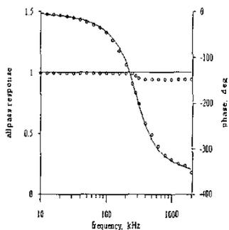
Fig. 5. The measured Allpass response with  $f_o=283\text{kHz}$  and  $Q=1$
