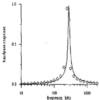
Fig. 4. The measured positive Bandpass response with  $f_o=283\text{kHz}$  and  $Q=10$
