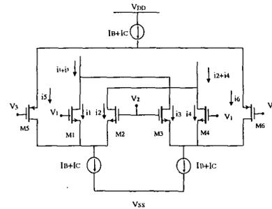
Fig.5 The proposed analog four-quadrant multiplier circuit.
