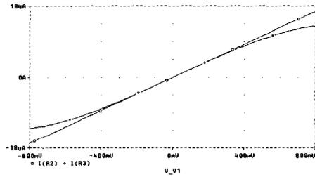
Fig.7 The I-V characteristics of the linearized LTP versus the ordinary LTP.
