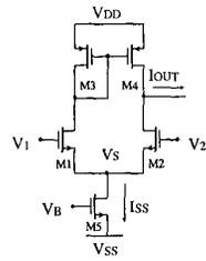
Fig.1 The ordinary LTP transistor circuit.
