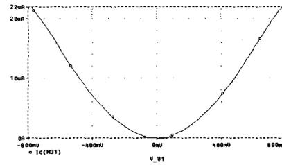
Fig.6 The I-V characteristics of the proposed squaring circuit.
