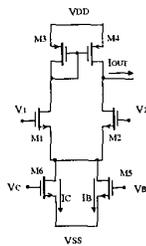
Fig.2 The linearized LTP transistor circuit.
