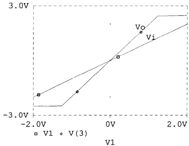
Fig.3(b) The output of the CFDDA voltage doubler.
