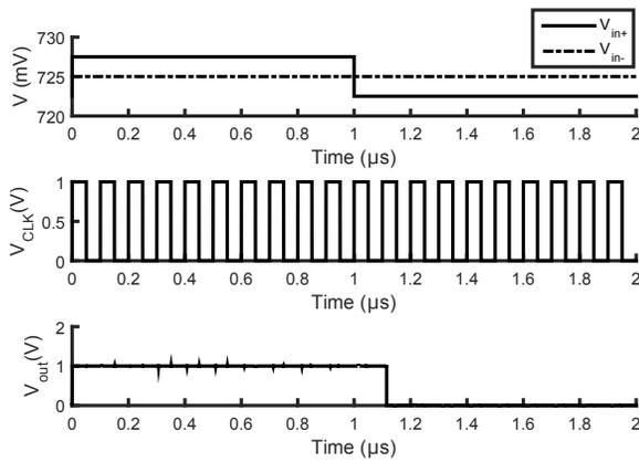
Fig. 4: Comparator Overdrive Recovery Test ( $V_{in} = 2$  mV and  $f_s = 10$  MHz)
