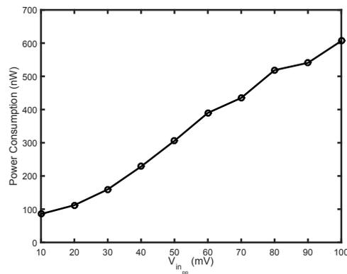
Fig. 7: Power Consumption versus  $V_{in,pp}$
