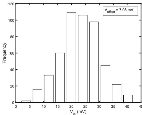
Fig. 5: Offset Voltage Monte-Carlo Simulation
