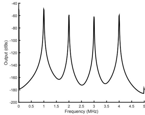
Fig. 6: Output Spectrum for Sinusoidal Input of 1 MHz Input Frequency
