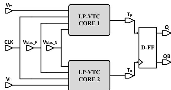
Fig. 1: Proposed Time-Domain Comparator Block Diagram
