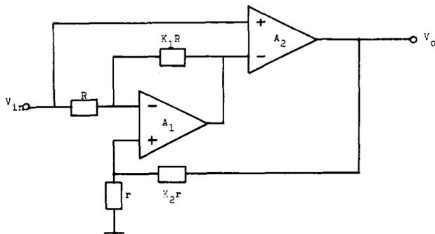
Fig. 2. The active compensated, noninverting VCVS.
