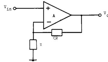
Fig. 1. The uncompensated, noninverting VCVS.
