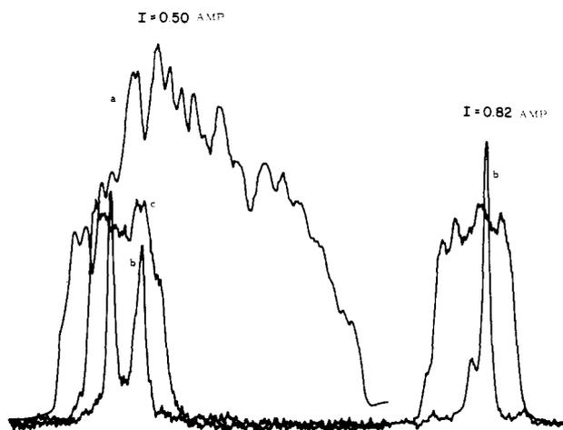
Fig. 2. (a) TDL radiation pattern. (b) TDL radiation pattern through pipe in one position. (c) TDL radiation pattern through pipe in orthogonal position.
