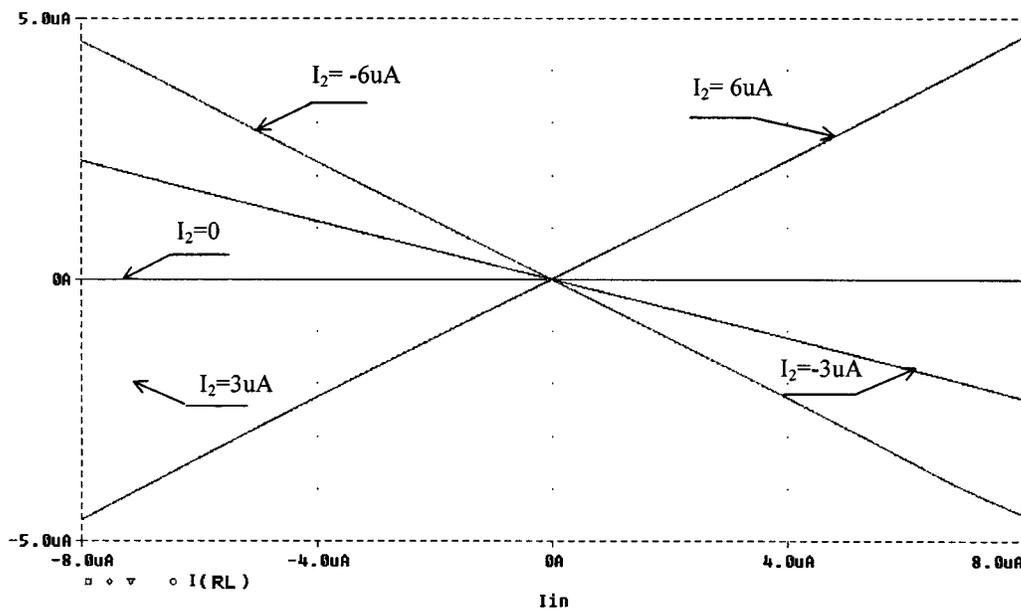
Fig. 8. DC simulation of the multiplier.
