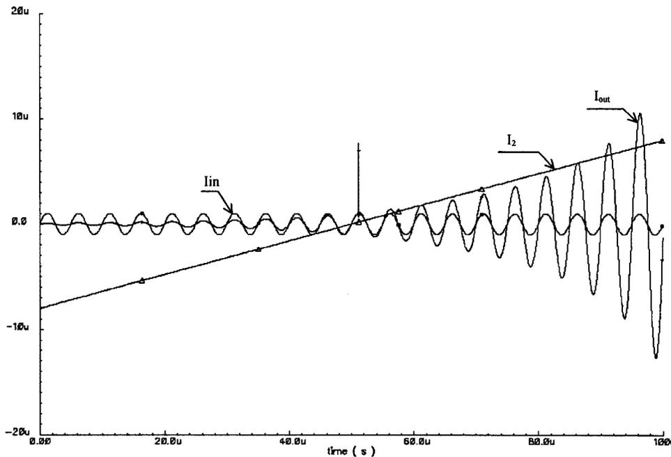
Fig. 15. Transient analysis of the overall circuit,  $I_{in}$  is a 200-kHz sinusoidal signal and  $I_2$  is a ramp.  $I_{out}$  is shown to have variable amplitude.
