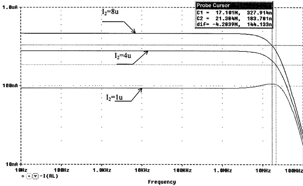
Fig. 9. Frequency response of the multiplier for three different gain values.
