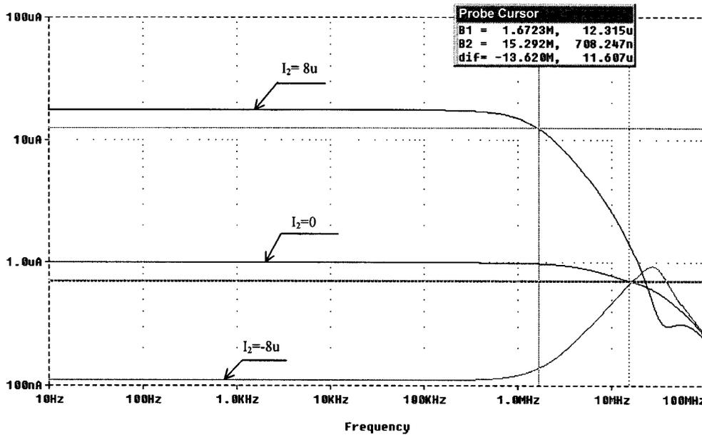
Fig. 14. Frequency response of the output current for three different gain values.
