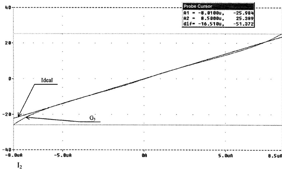
Fig. 13. Combined approximation function ( $G_3$ ) and an ideal exponential function versus control signal  $I_2$ .
