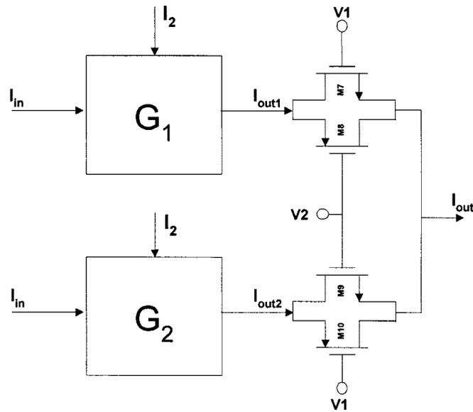
Fig. 11. Block diagram to realize  $G_3$ .
