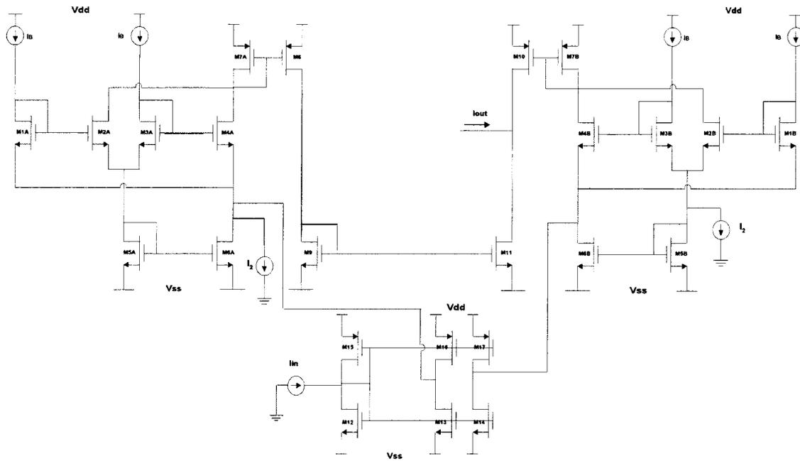
Fig. 7. The multiplier circuit introduced in [10].
