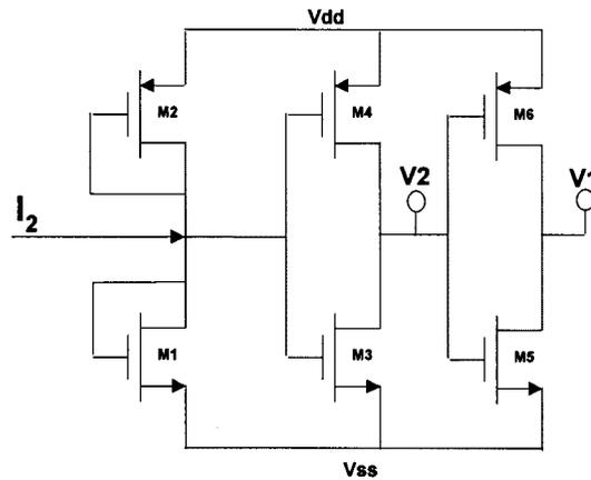
Fig. 12. Circuit used to generate the control voltages  $V_1$  and  $V_2$  to be used in the block diagram of Fig. 11.
