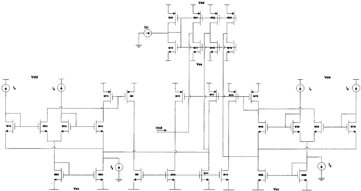
Fig. 10. Circuit used for implementing  $G_1$  and  $G_2$ .
