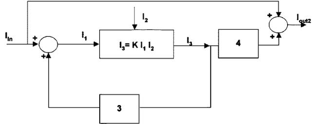
Fig. 6. Block diagram for the realization of  $G_2$ .
