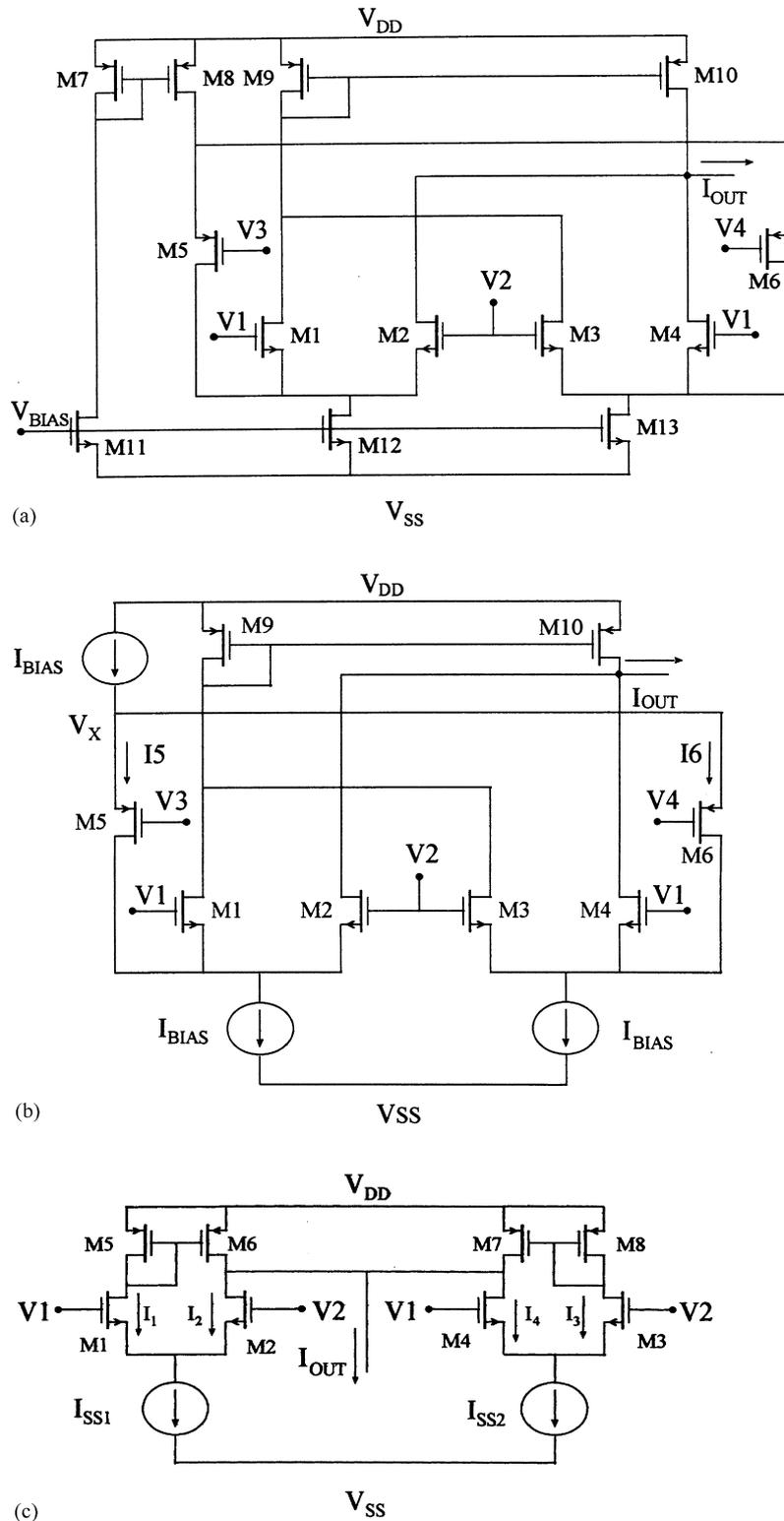
Fig. 10. (a) The voltage-controlled transconductor proposed in [1]. (b) The modified transconductor (a) showing the equivalent biasing currents. (c) The equivalent LTP circuit of the circuit in (a).
