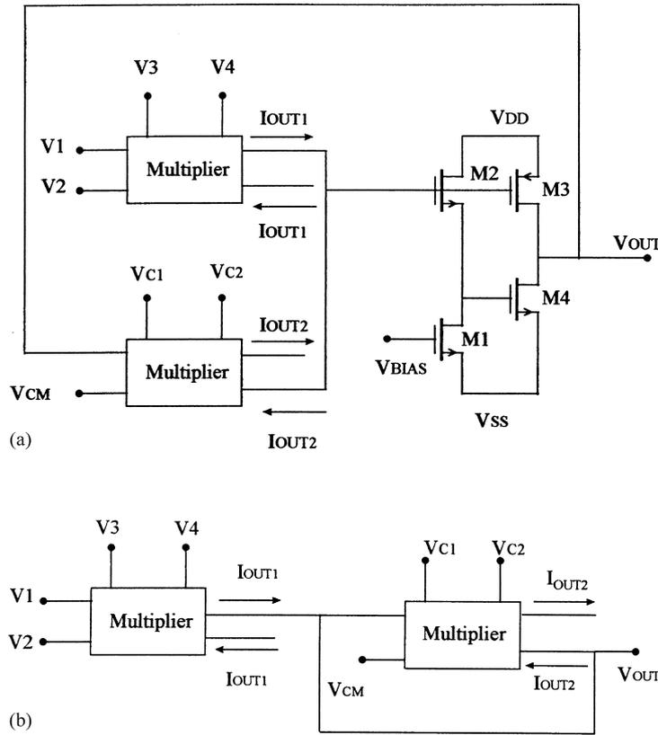
Fig. 14. The proposed multiplier divider based on CMOS voltage-controlled transconductor.
