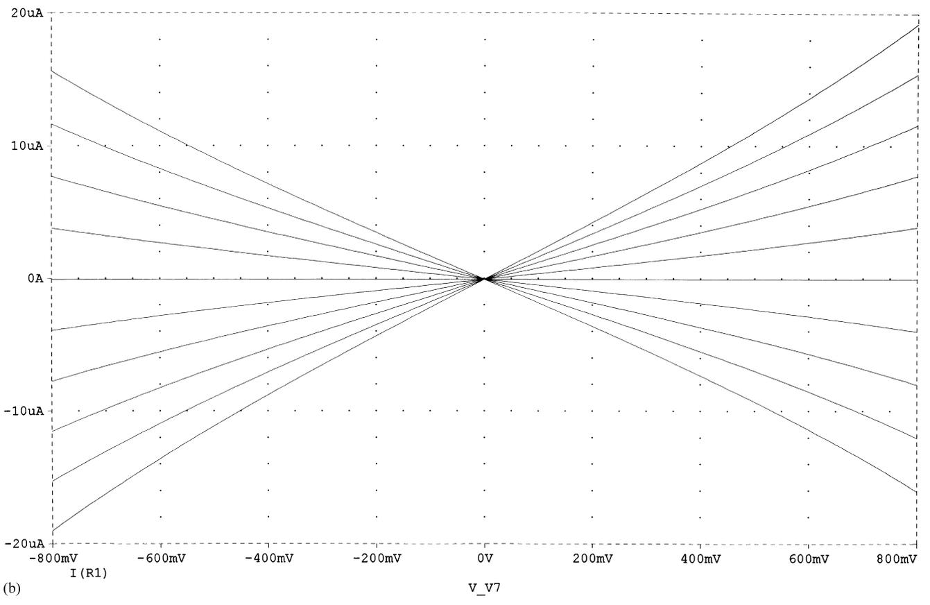
Fig. 12. (a) The  $I$ - $V$  characteristics of the voltage-controlled CMOS transconductor proposed in [1] for different values of the control voltage. (b) The  $I$ - $V$  characteristics of the voltage-controlled CMOS BOTA for different values of the control voltage.
