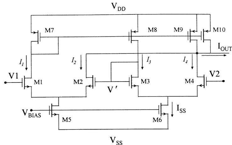
Fig. 3. The normalized two stage ELTP CMOS transconductor.
