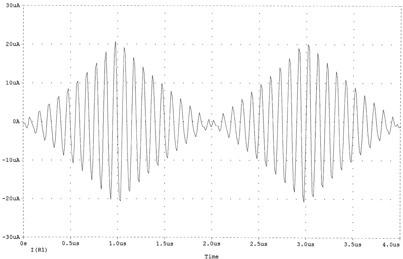
Fig. 13. The Transient analysis of the output current of the voltage-controlled CMOS BOTA resulting from the multiplication of two differential input voltages.
