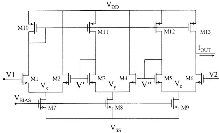
Fig. 4. The three stage ELTP CMOS transconductor.
