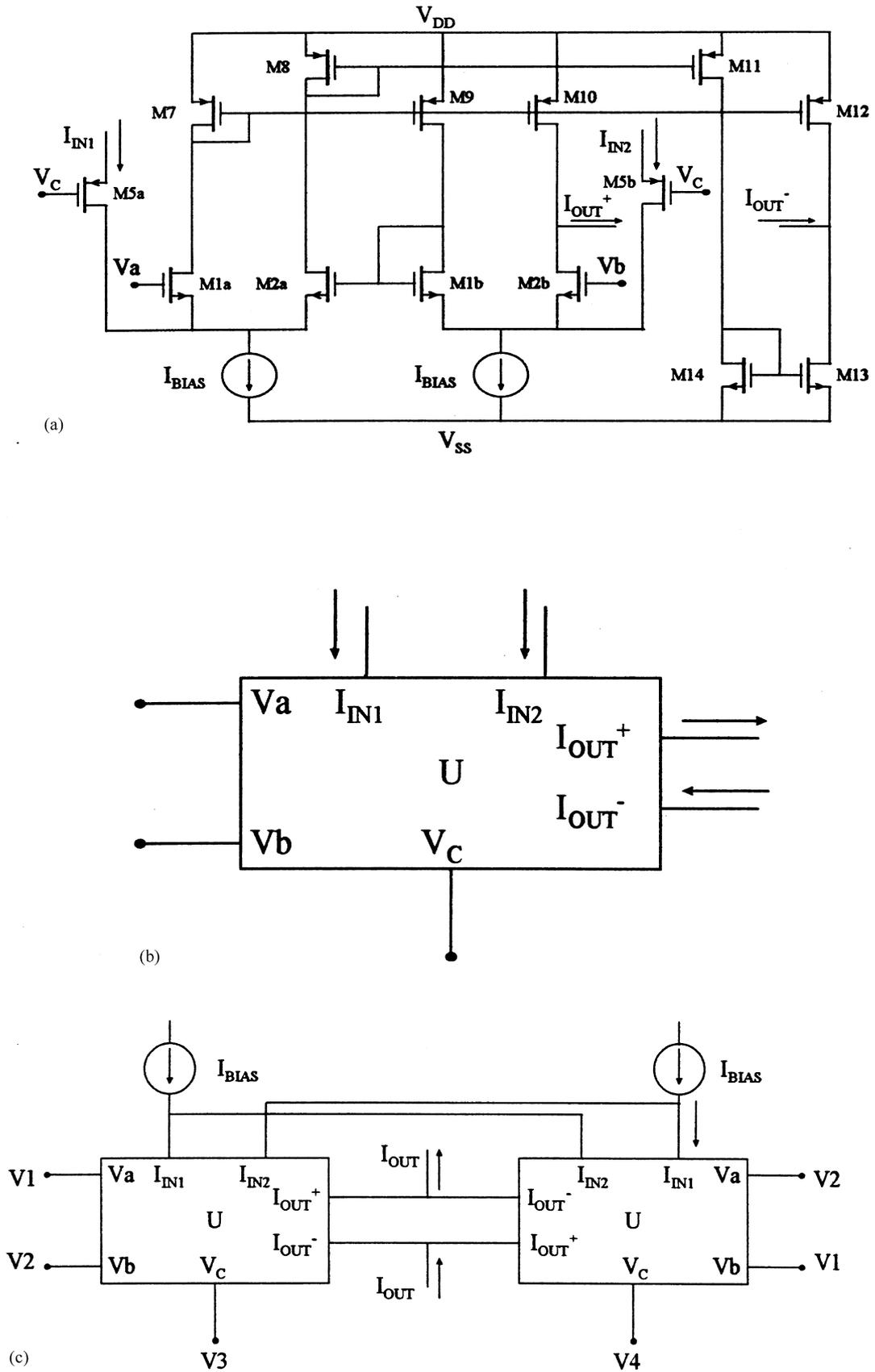
Fig. 11. (a) The equivalent LTP circuit of one pair of NMOS transistors of voltage-controlled transconductor proposed in [1]. (b) The equivalent building block of (a). (c) The proposed voltage-controlled CMOS BOTAs.
