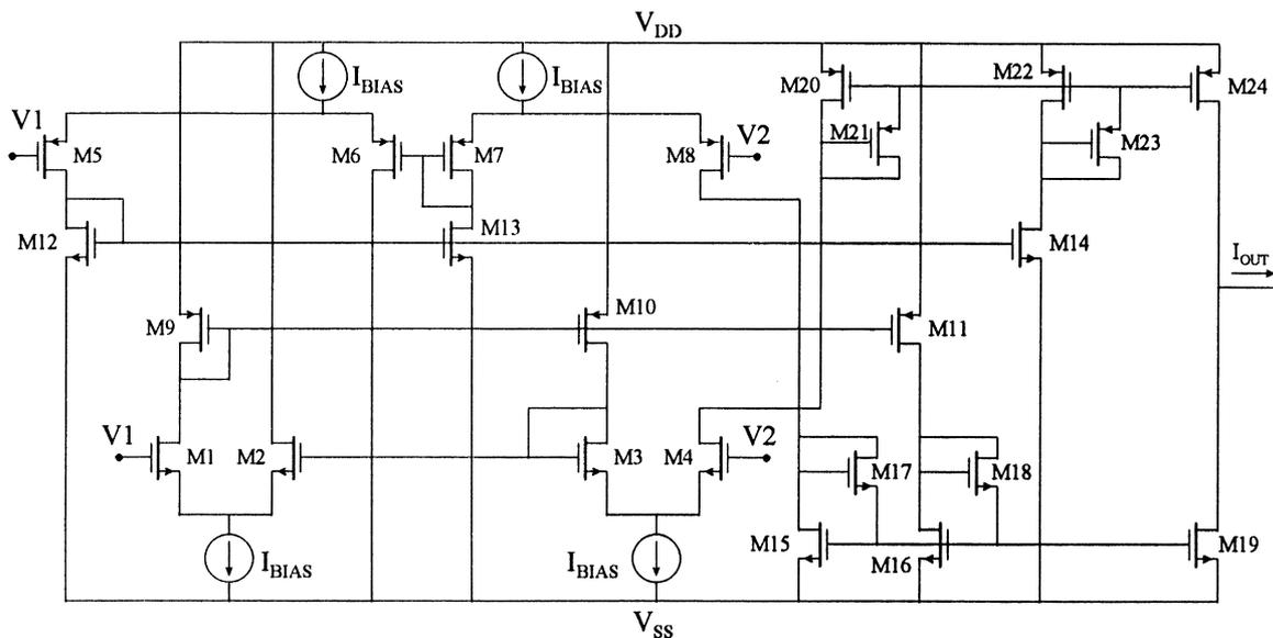
Fig. 17. The proposed rail-to-rail CMOS transconductor.
