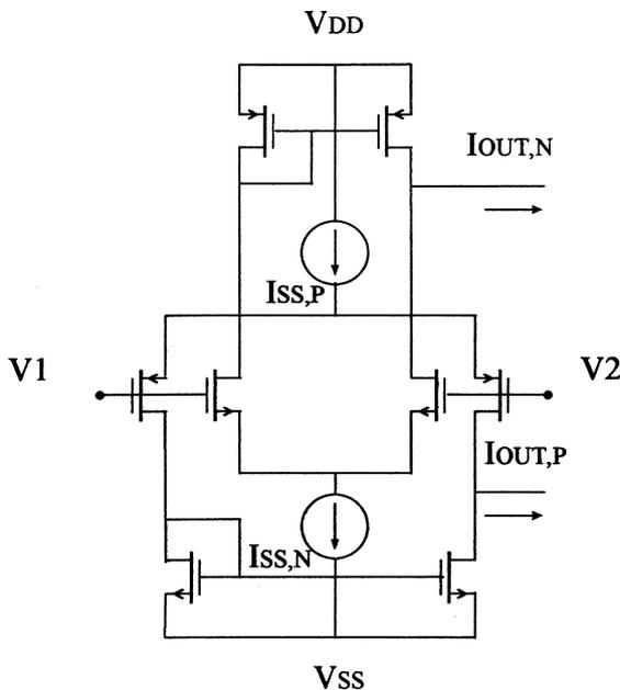
Fig. 15. The complementary differential input stage with active load.
