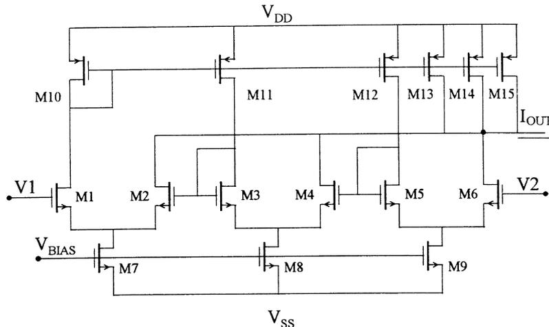
Fig. 5. The normalized three stage ELTP CMOS transconductor.
