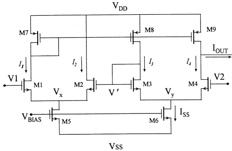
Fig. 2. The two stage ELTP CMOS transconductor.
