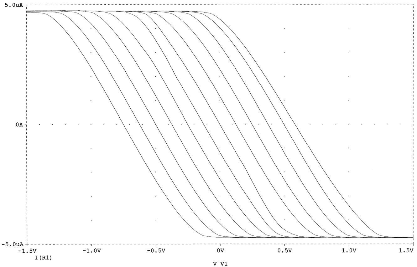
Fig. 18. The  $I$ – $V$  characteristics of the CMOS rail-to-rail transconductor.
