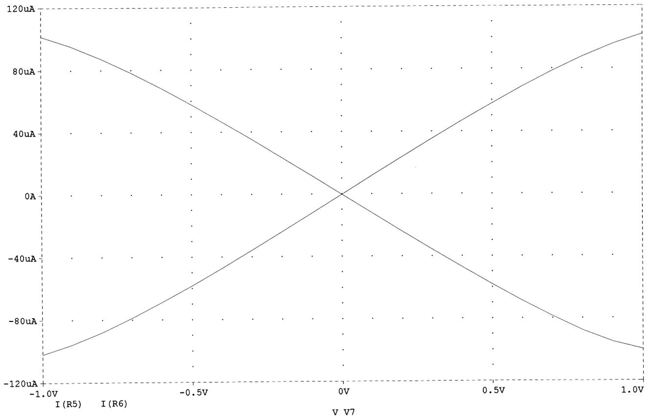
Fig. 9. The  $I$ - $V$  characteristics of the CMOS BOTA.
