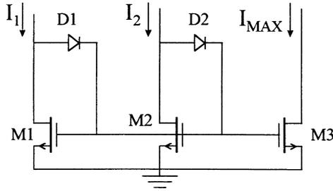
Fig. 16. The maximum circuit used to extract the maximum of two currents [12].
