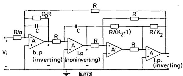
Fig. 2 Improved Tow-Thomas biquad filter suitable for high  $Q$  and high frequency. Magnitude of gain at  $\omega_0$  at each of three outputs =  $aQ_0$
