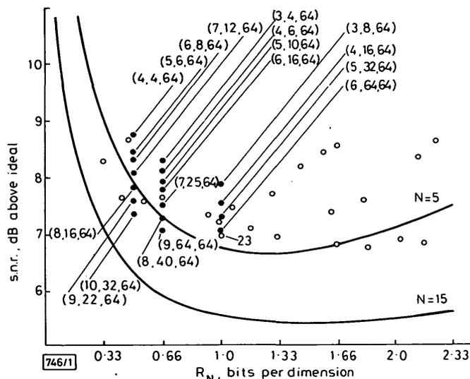
**Fig. 1** Performances of some  $(N, M, 64)$  codes (denoted by ●) and permutation modulation codes<sup>3</sup> (denoted by ○) for word error probability  $P_e = 10^{-5}$
