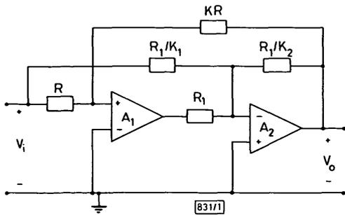
Fig. 1 Novel variable-phase inverting amplifier
