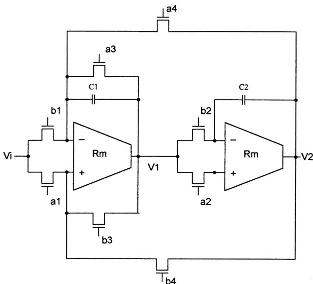
Fig. 9. The TT biquad circuit.
