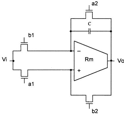
Fig. 8. Generalized voltage-mode integrator.
