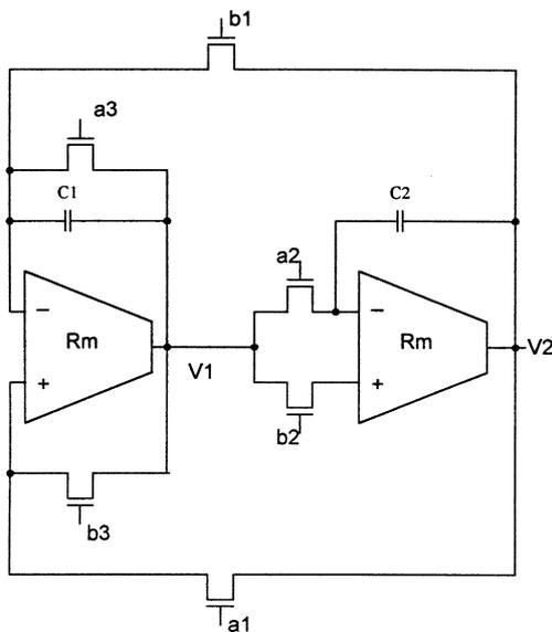
Fig. 16. Quadrature oscillator circuit.
