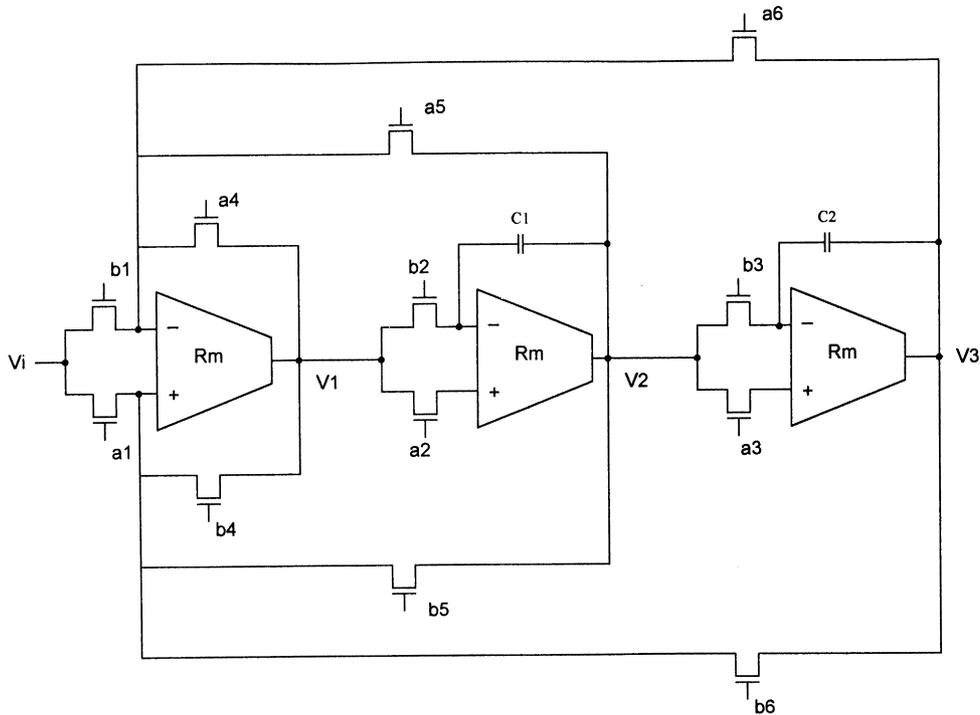
Fig. 11. The KHN biquad circuit.
