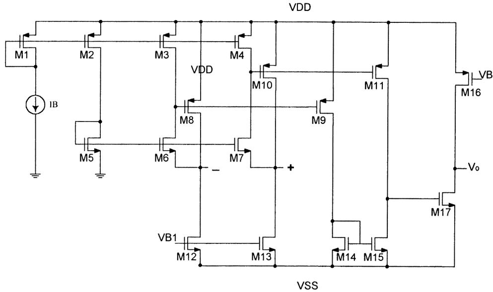
Fig. 1. Proposed CMOS realization of the OTRA.
