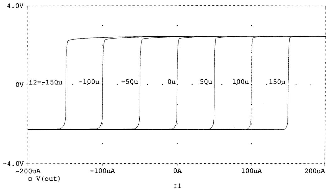
Fig. 2. Output voltage of the OTRA.
