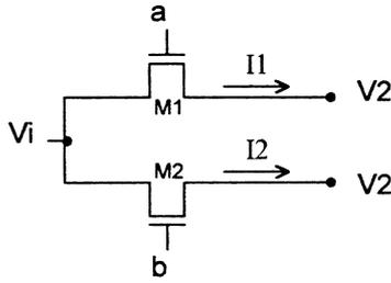
Fig. 3. Non-linearity cancellation in two matched NMOS transistor circuit.
