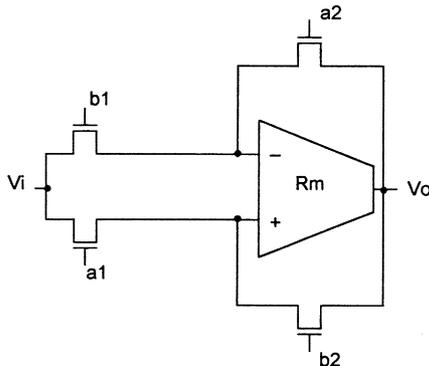
Fig. 4. OTRA-based VCVS.
