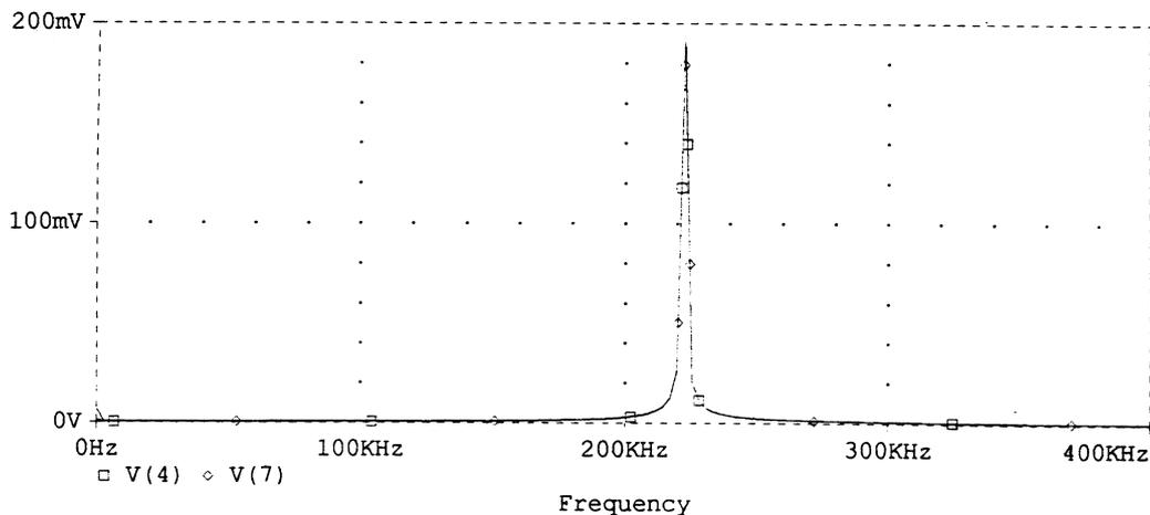
Fig. 18. Oscillator frequency spectrum.
