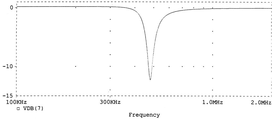
Fig. 15. Band stop response of the universal filter.
