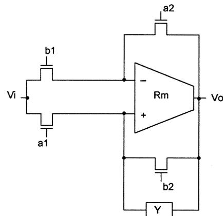
Fig. 7. Passive compensated VCVS.
