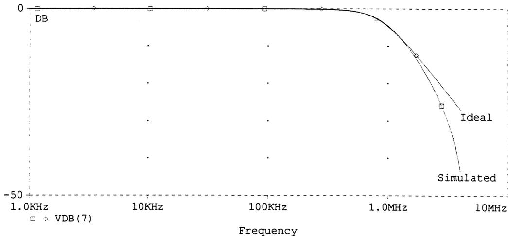
Fig. 10. Ideal and simulated responses for a Butterworth lowpass filter.
