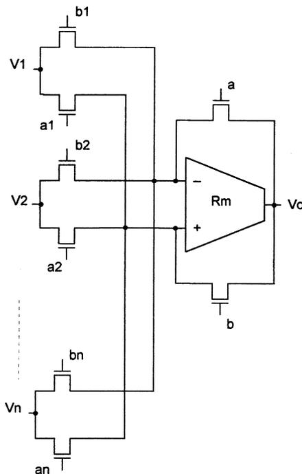
Fig. 6. Weighted summer OTRA-based circuit.
