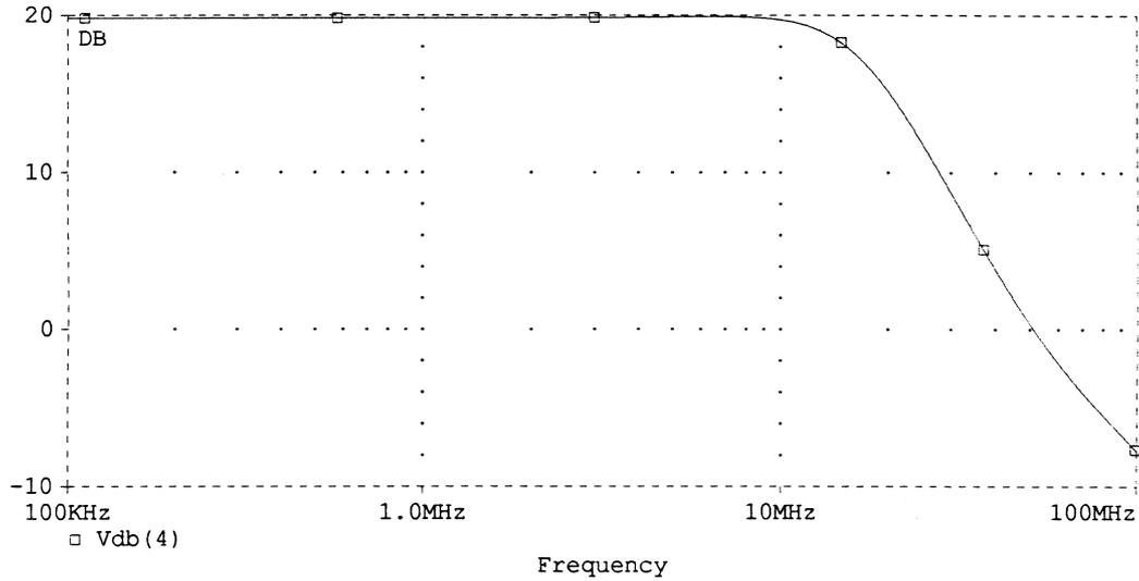
Fig. 5. Frequency spectrum of the VCVS with gain = 10.
