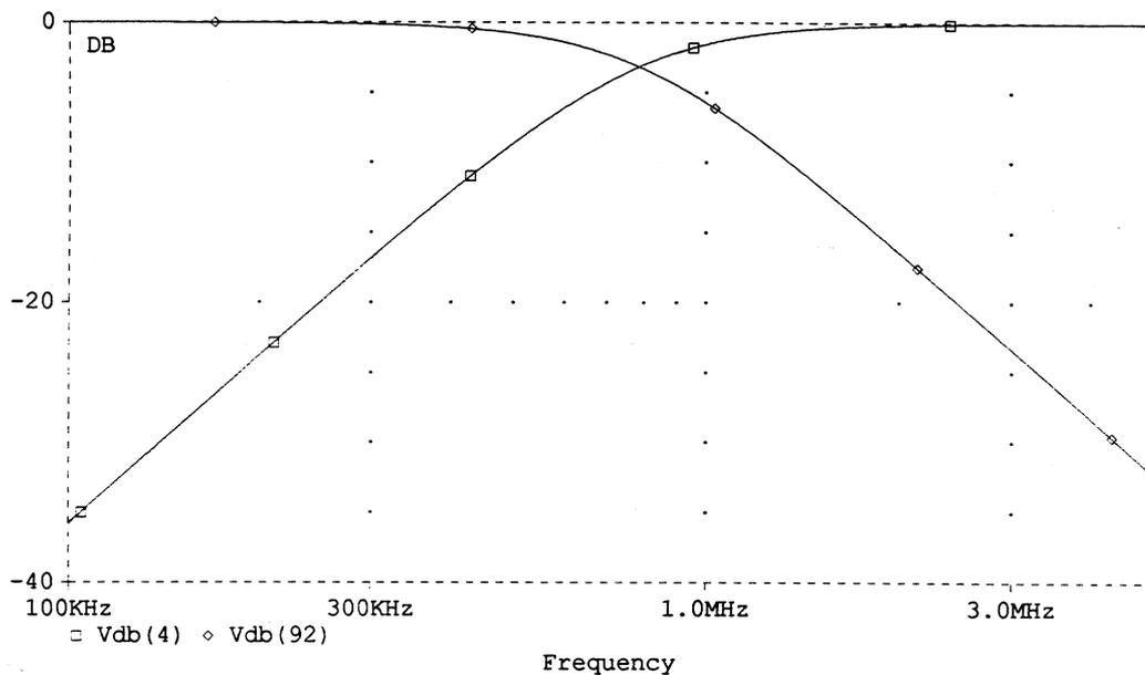
Fig. 12. Highpass and lowpass responses of the KHN biquad.
