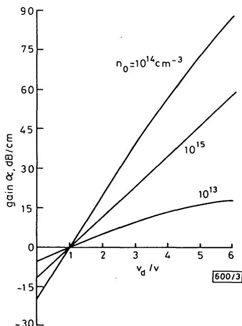
**Fig. 3** Amplification characteristics of m.e.l.w.s when diffusion included
