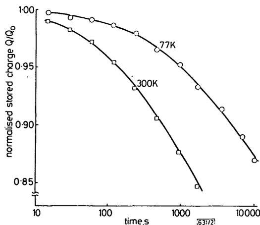
**Fig. 2** Normalised decay of stored charge at room temperature and 77 K
