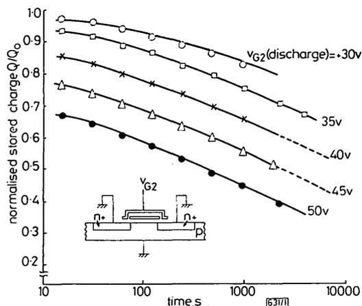
**Fig. 1** Normalised room-temperature decay of stored charge with the top gate voltage as a parameter
